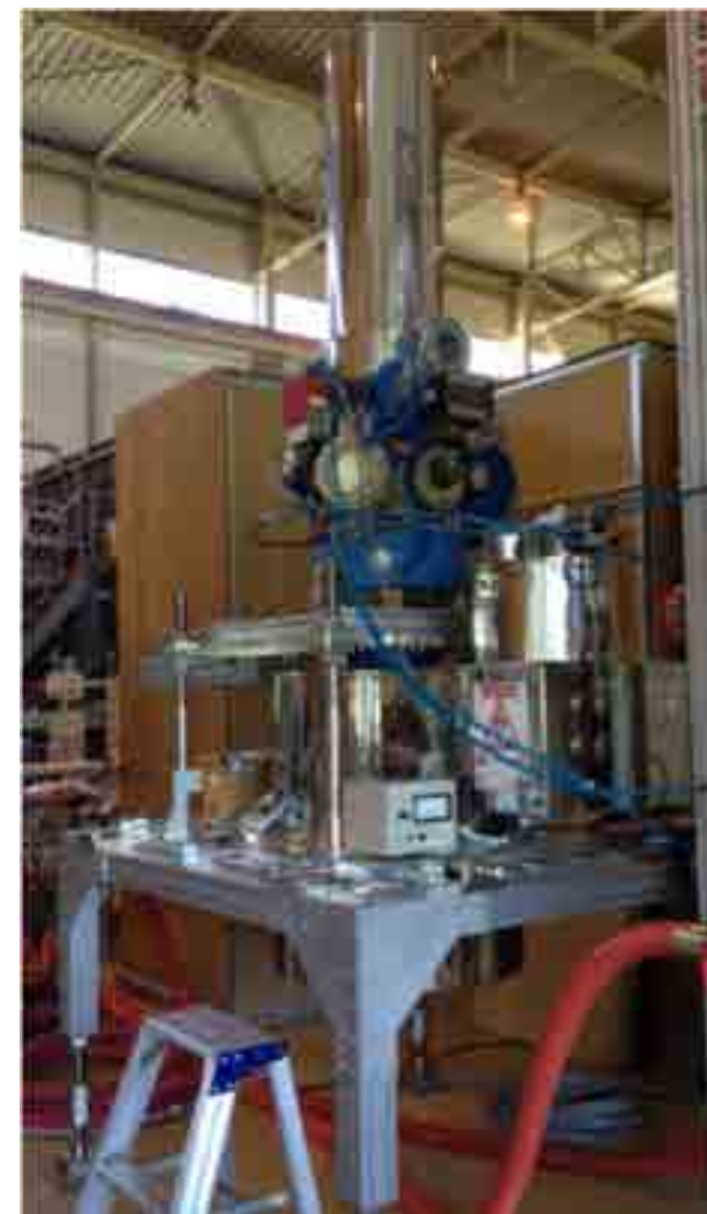
7T240 SCM installed in QST
