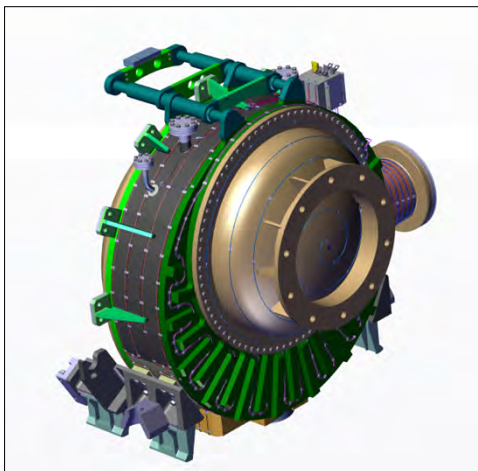
Figure 10: General view of The VVPSS box Blank Flange
