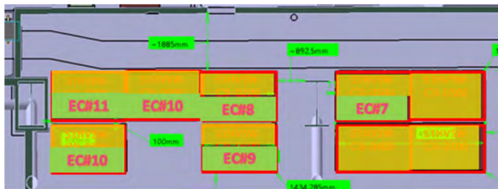
Figure 4-2 ECH switchgear layout in B15-L1-03
