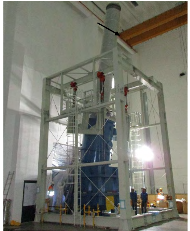
Gate type jig 5.6 x 5.7 x 8.9, 14.5t (L x W x H, m)
