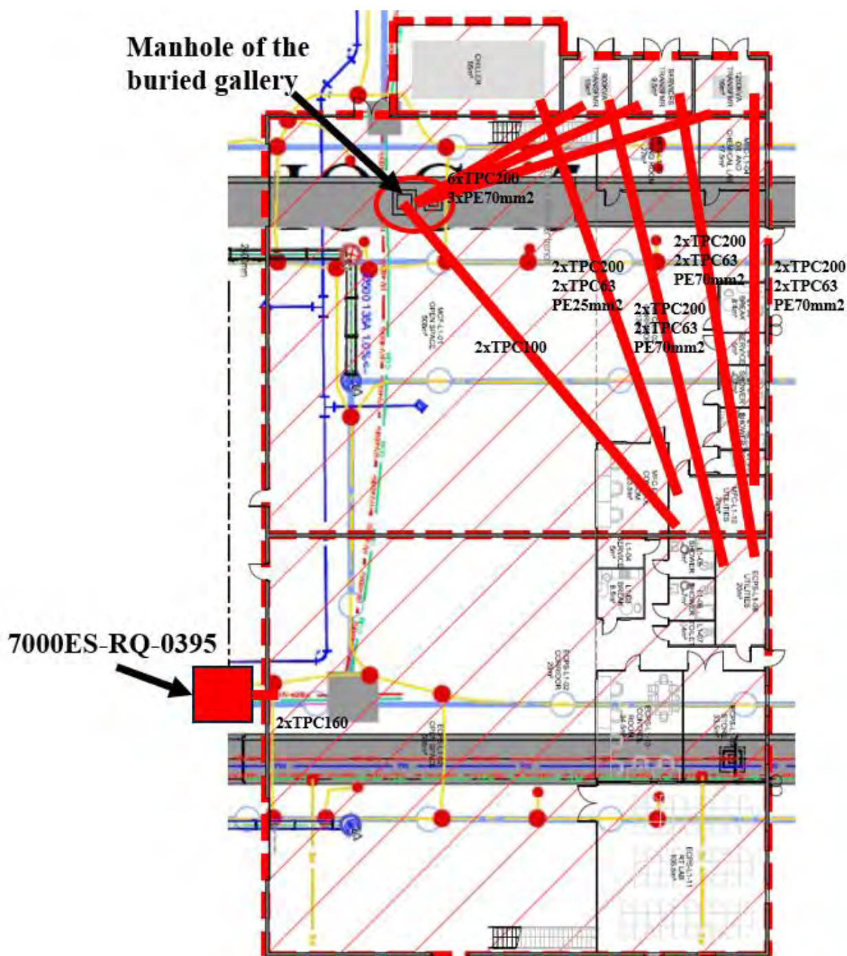
Figure 3 - Simplified plan of HV and LC ducts installation
