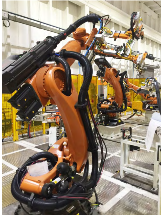
Figure 11: Example of cable management solution.
