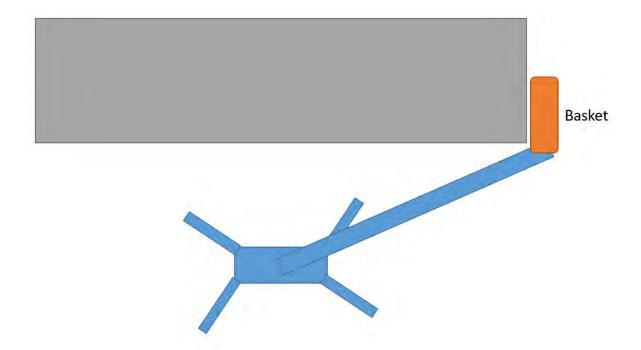
To extend the working range, and unless the boom has an additional articulation before the basket, it is considered that the basket is mounted on the short side to be able to work along the side. As such the tenderer shall propose a basket optimizing this possibility and the related impact on the working load and cost of the e-cherry picker. With extra articulation, the relevant load curves shall be presented, giving the remaining load capacity at the basket.
