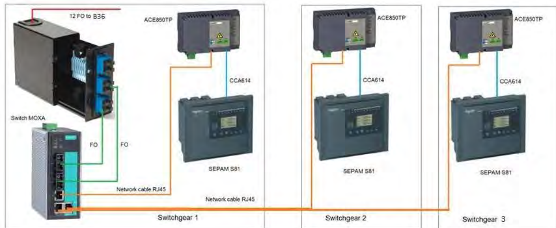
Overview of the sepam architecture (22kV+15kV)
