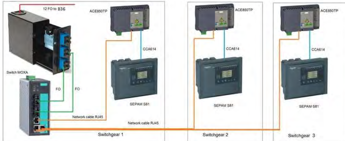
Overview of the sepam architecture (22kV+15kV)
