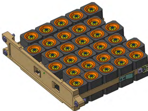
Figure 5-1 - Boron carbide block arrangement (B4C) in shielding tray
