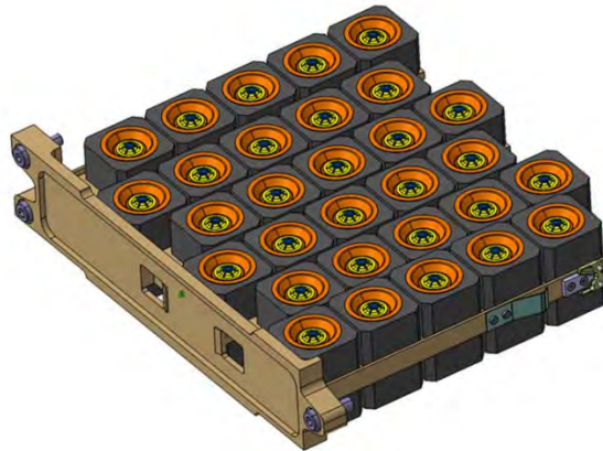
Figure -3 Boron carbide block arrangement ( B_4C ) in shielding tray
