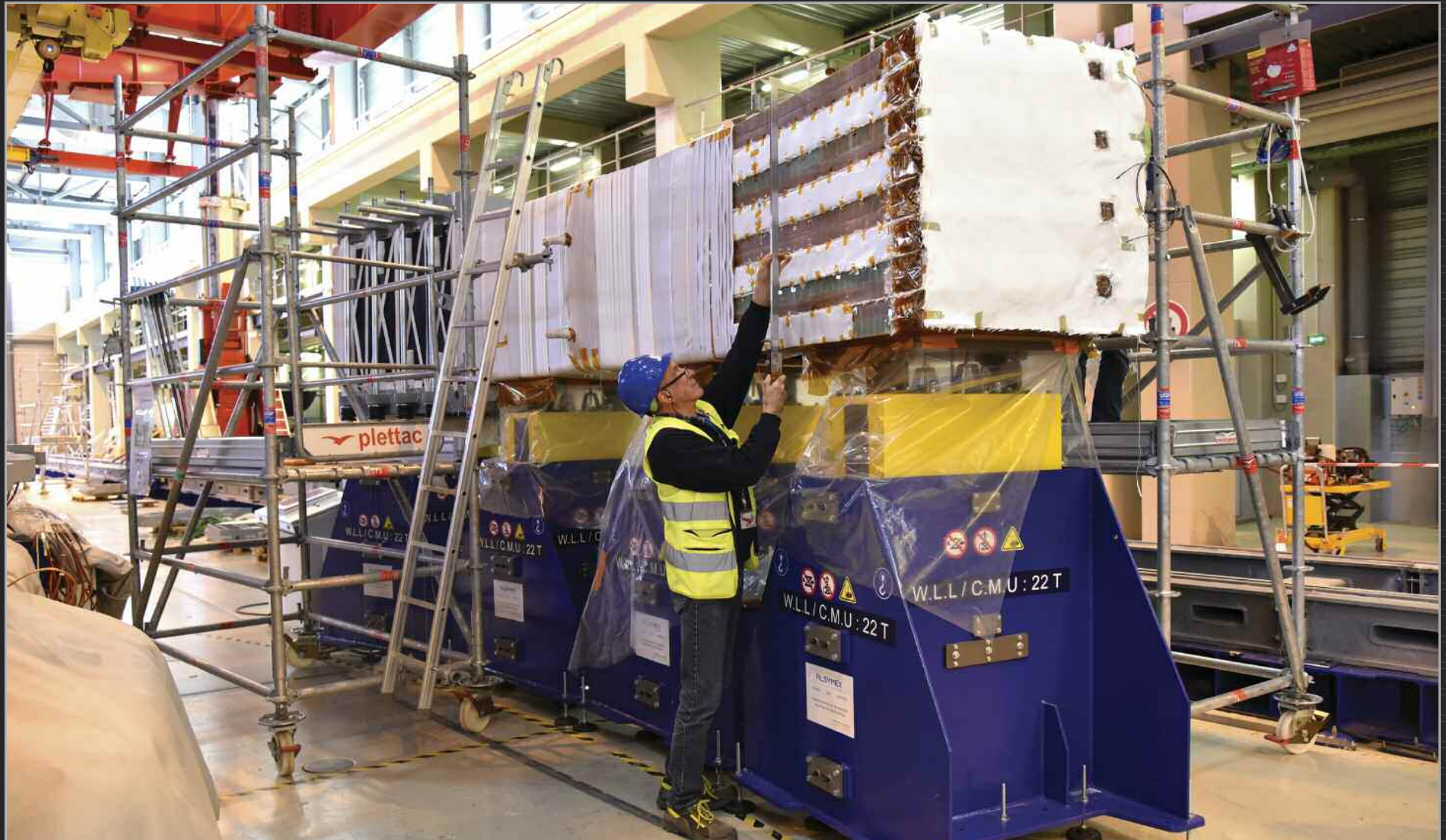
This segment of mockup coil faithfully mimics poloidal field coil #5 (PF5) and its eight stacked double pancakes. It is used in 2019 to test winding pack impregnation, before the operation is carried out on the production coil. March 2019
