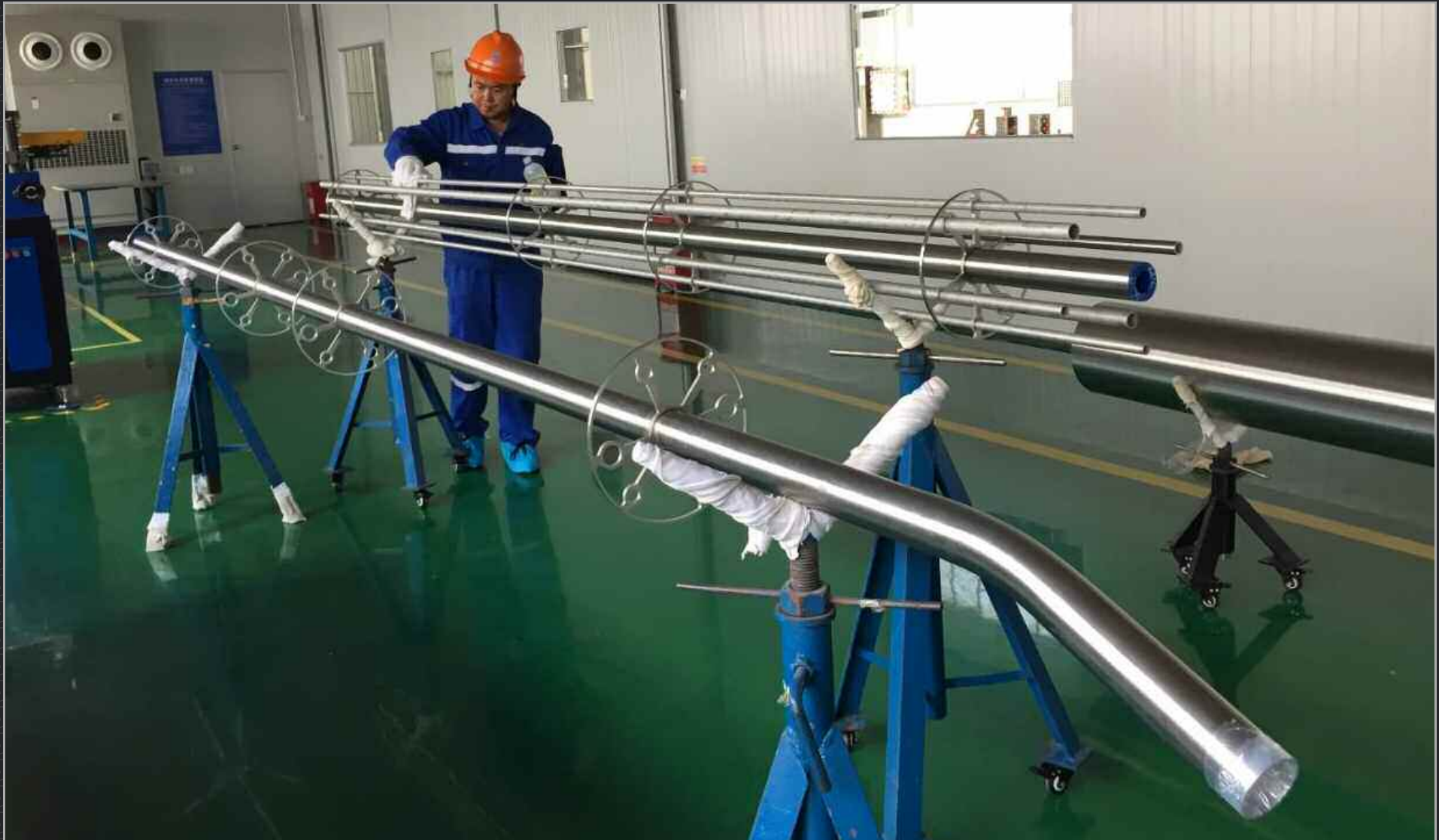
Different gas species from the Tritium Plant will be delivered to the fuelling, neutral beam and disruption mitigation systems via a gas distribution manifold system. The assembly of the first manifold spool is ongoing, including the process pipes, guard pipe, evacuation pipe and inner supports.
