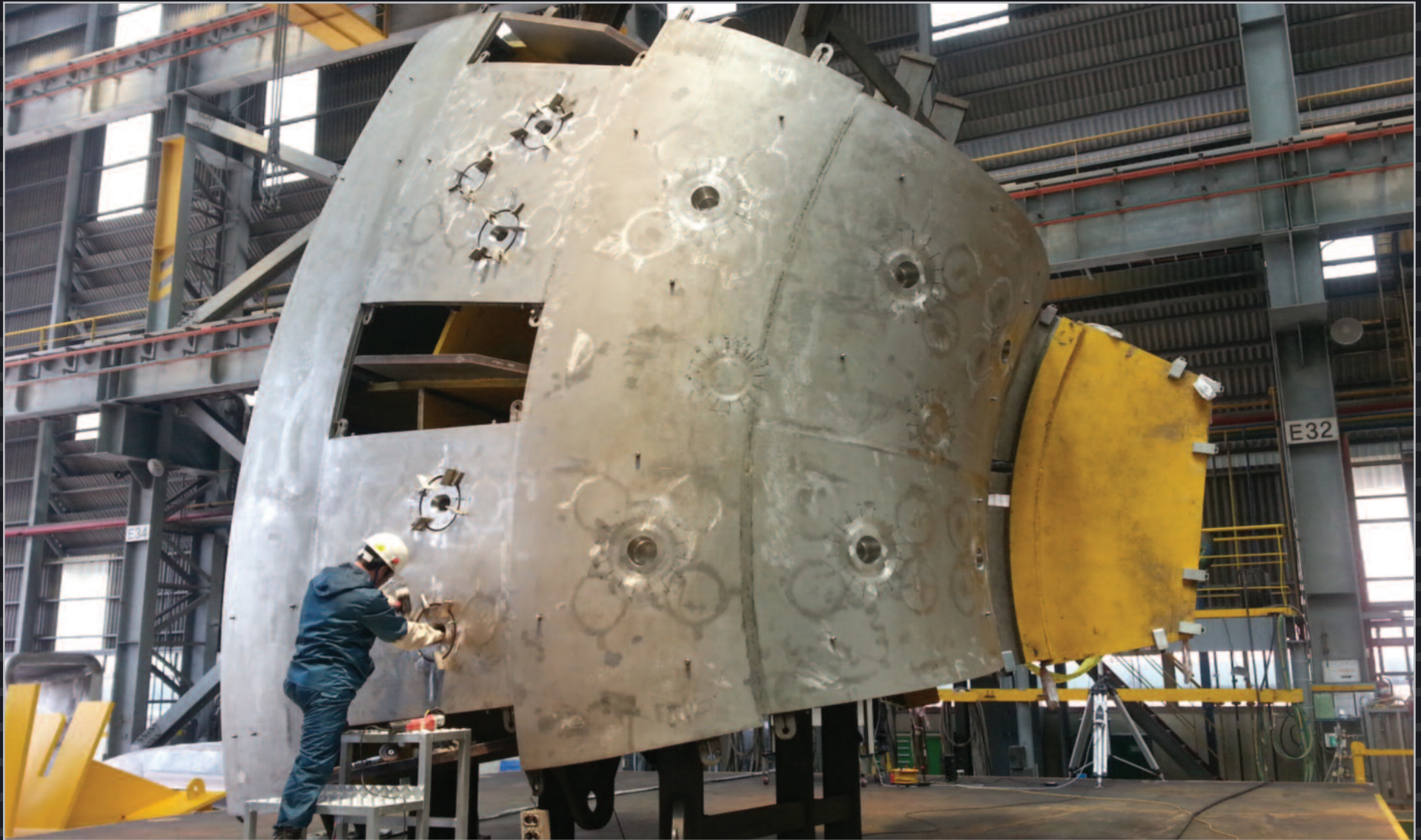
Manufacturing of the ITER vacuum vessel is underway in Korea, which is responsible for procuring two sectors out of nine. Pictured: welding operations at Hyundai Heavy Industries in Ulsan on an inner shell upper section – only a small part of one sector.
