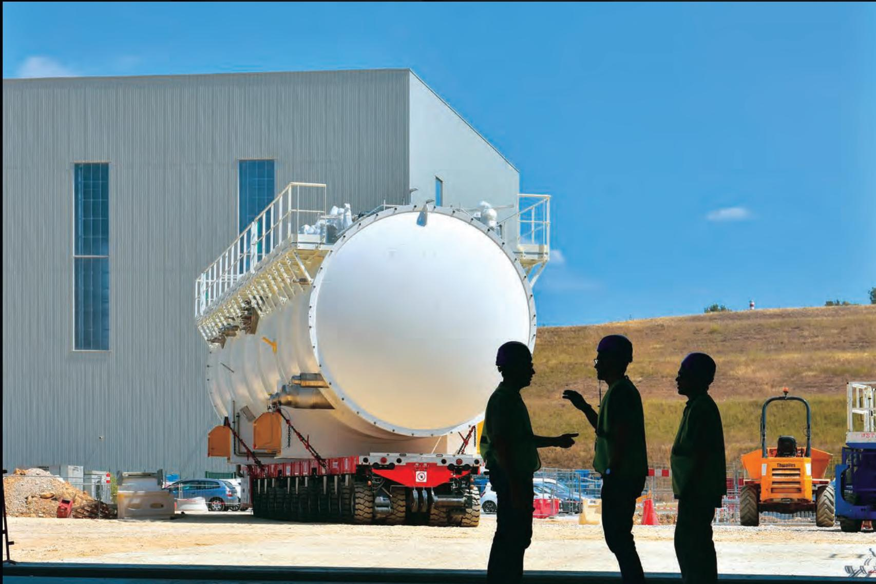
Manufactured in France by Air Liquide, this helium "cold box" – installed with two others in the cryoplat during the year – will provide insulation for the key components of the liquid helium plants.
