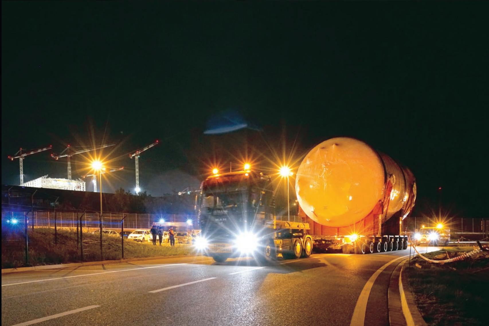
The first of five drain tanks for the tokamak cooling water system arrives from the United States.
