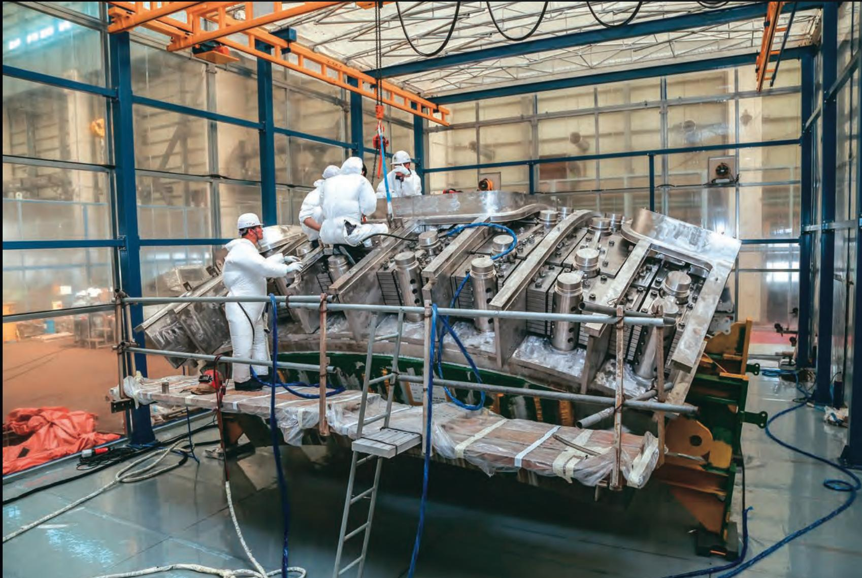
Hyundai Heavy Industries is manufacturing four of ITER's nine vacuum vessel sectors. Pictured: technicians are inserting neutron shielding blocks into one of four sector #6 segments.
