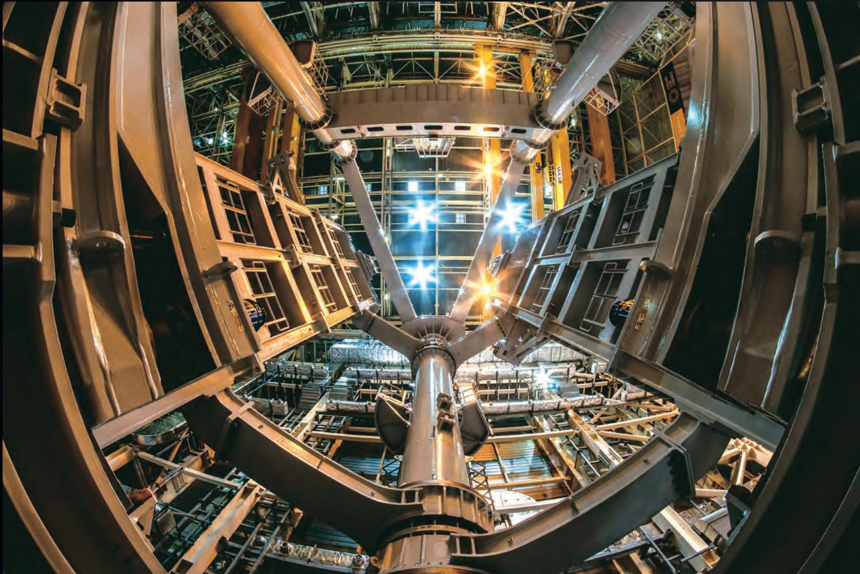
The sector sub-assembly tools that will permit the creation of 1,350-tonne vacuum vessel sub-assemblies, or "modules," weigh 800 tonnes and stand 22 metres tall. Pictured here is tool SSAT-1, supplied by Korea, that will soon have an identical twin in the Assembly Hall.
