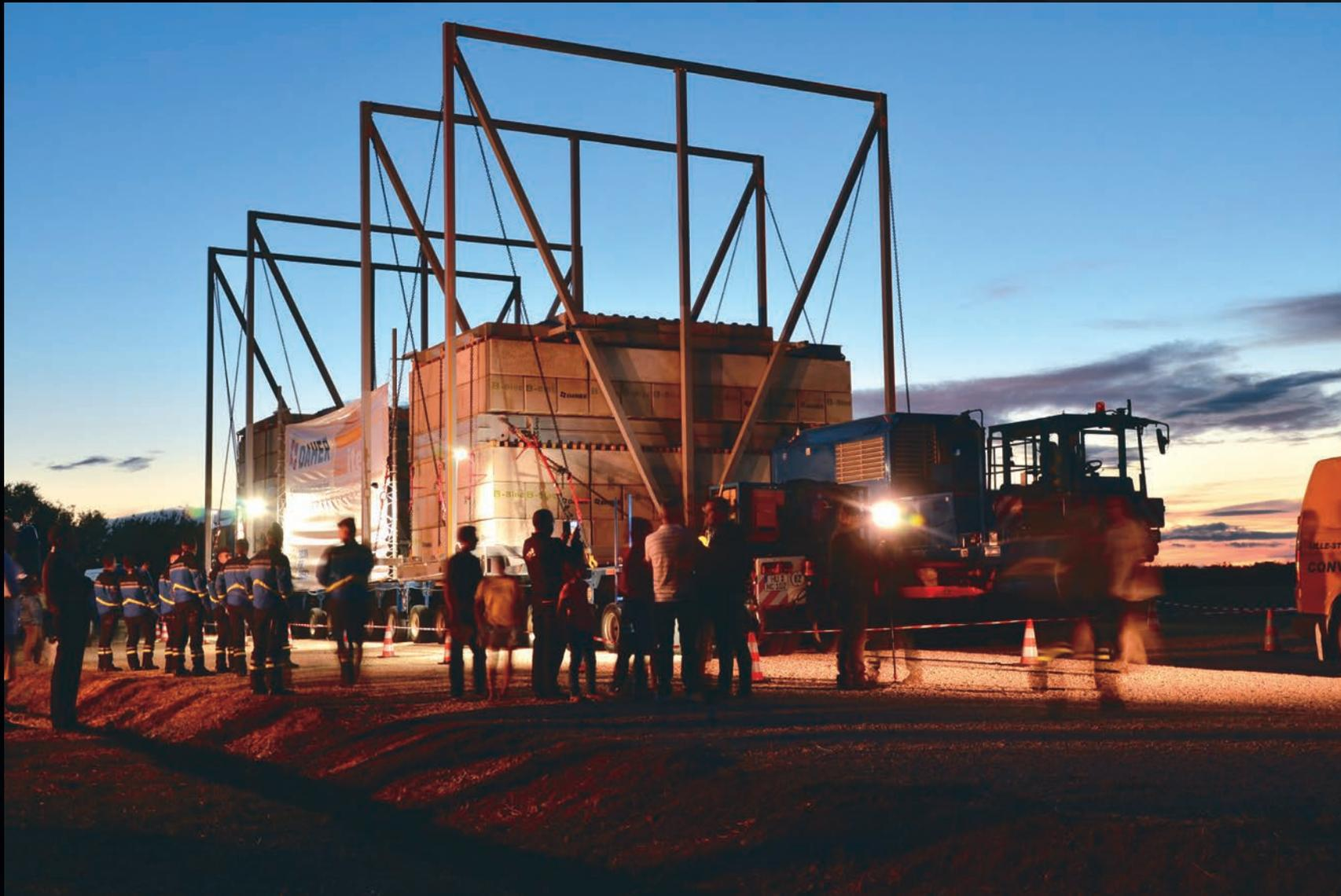
The road itinerary between the Mediterranean coast and the ITER site—the "ITER itinerary"—is tested with a 600-tonne load before the arrival of the first ITER components.
