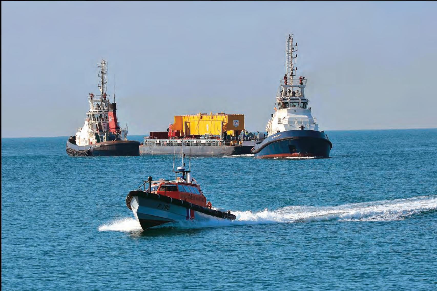
Pushed and pulled by powerful tugs and escorted by a patrol boat of the French Gendarmerie Maritime, the barge and its load (trailer plus a 155-tonne girder) approaches the entrance of the narrow channel that leads into the inland sea Étang de Berre.
