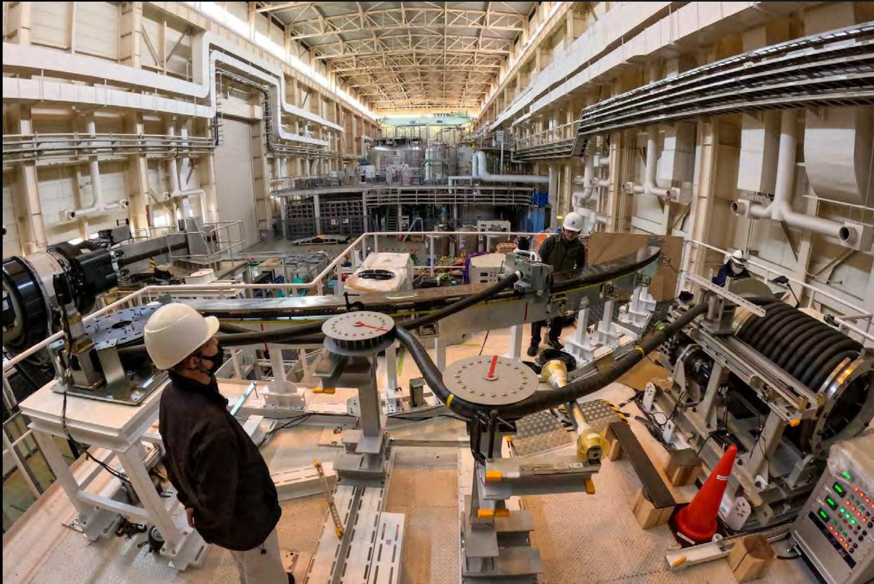
Captions □ To develop composite cable feeding control technology and cable guide mechanism for cable handling equipment, a mock-up test rig was fabricated and completed on March 31, 2023. Test is currently ongoing to reflect the results to the design.
