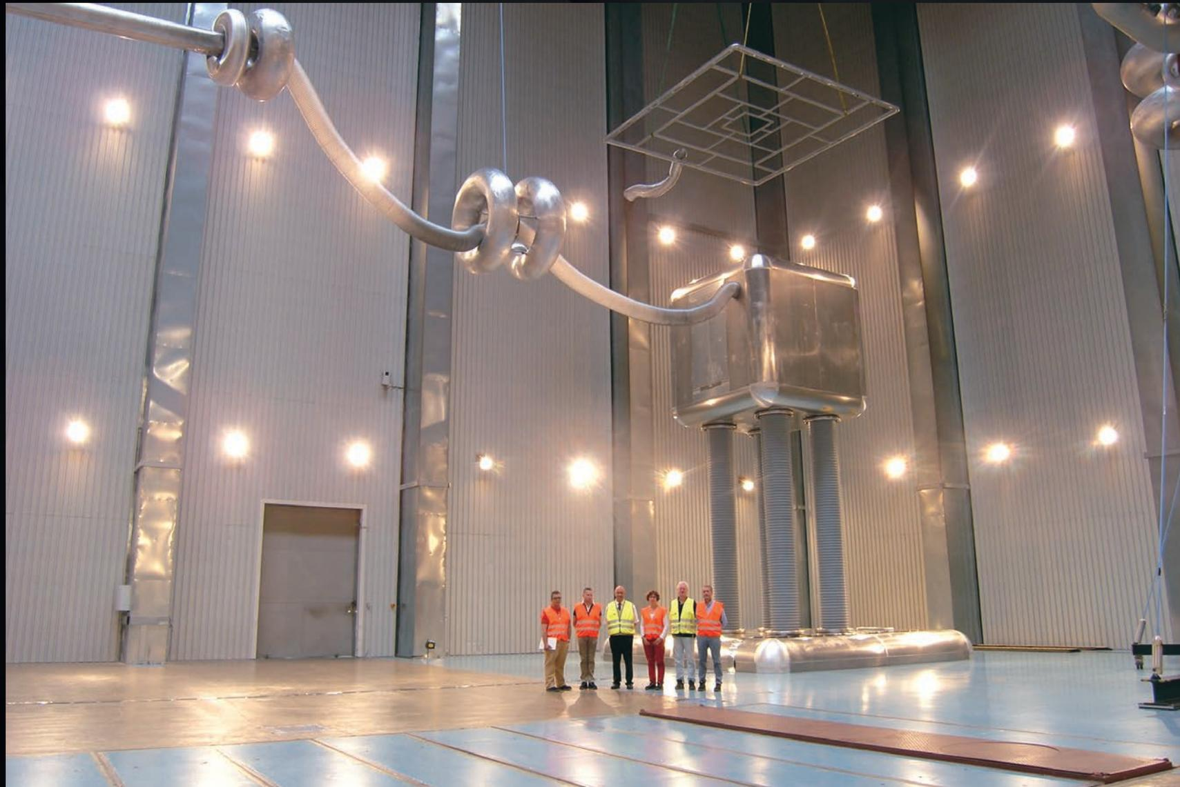
Six metres overhead, the mockup of a high voltage deck is tested successfully in a laboratory at HSP GmbH, Germany. The cube is 1/15th of the size of the deck that will be integrated into the MITICA testbed, currently under construction at the ITER Neutral Beam Test Facility in Padua, Italy.
