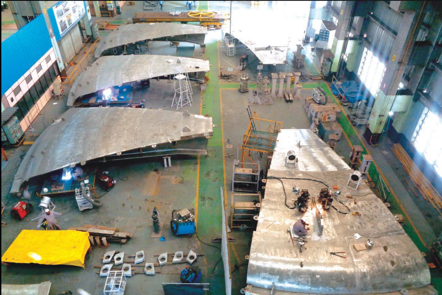
At the Larsen & Toubro factory in Hazira, India, elements of the cryostat top lid are in fabrication. When completed, they will be sent to the Indian Domestic Agency's workshop at ITER for assembly.
