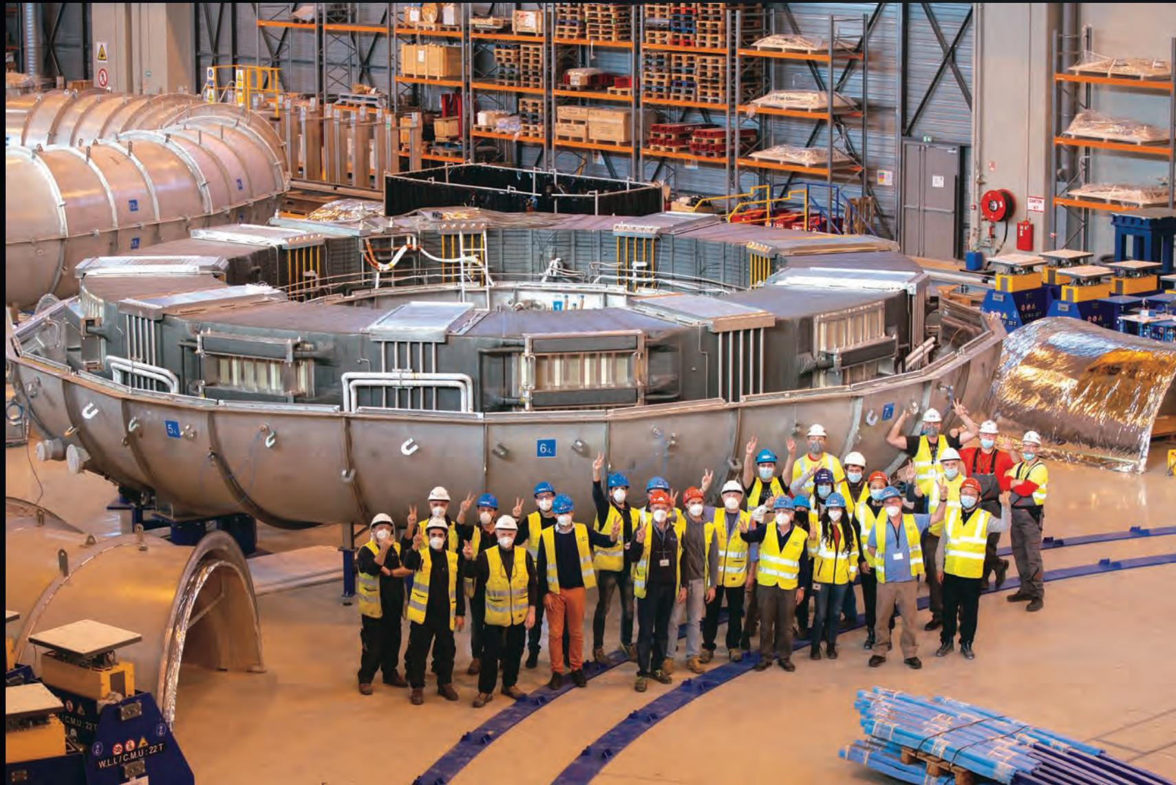
The first poloidal field coil completes all testing in December. Representatives of the European Domestic Agency Fusion for Energy, manufacturer ASIPP from China, and ASC Superconductors celebrate in front of the vacuum chamber where poloidal field coil #6 spent three months in thermal testing.
