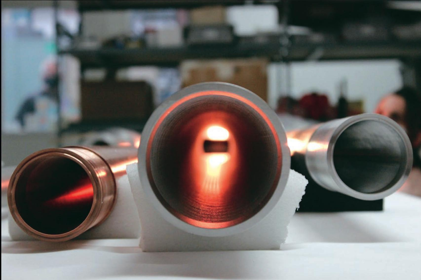
Qualification and fabrication of the electron cyclotron transmission line system is underway in the United States. Pictured are waveguide prototypes.
