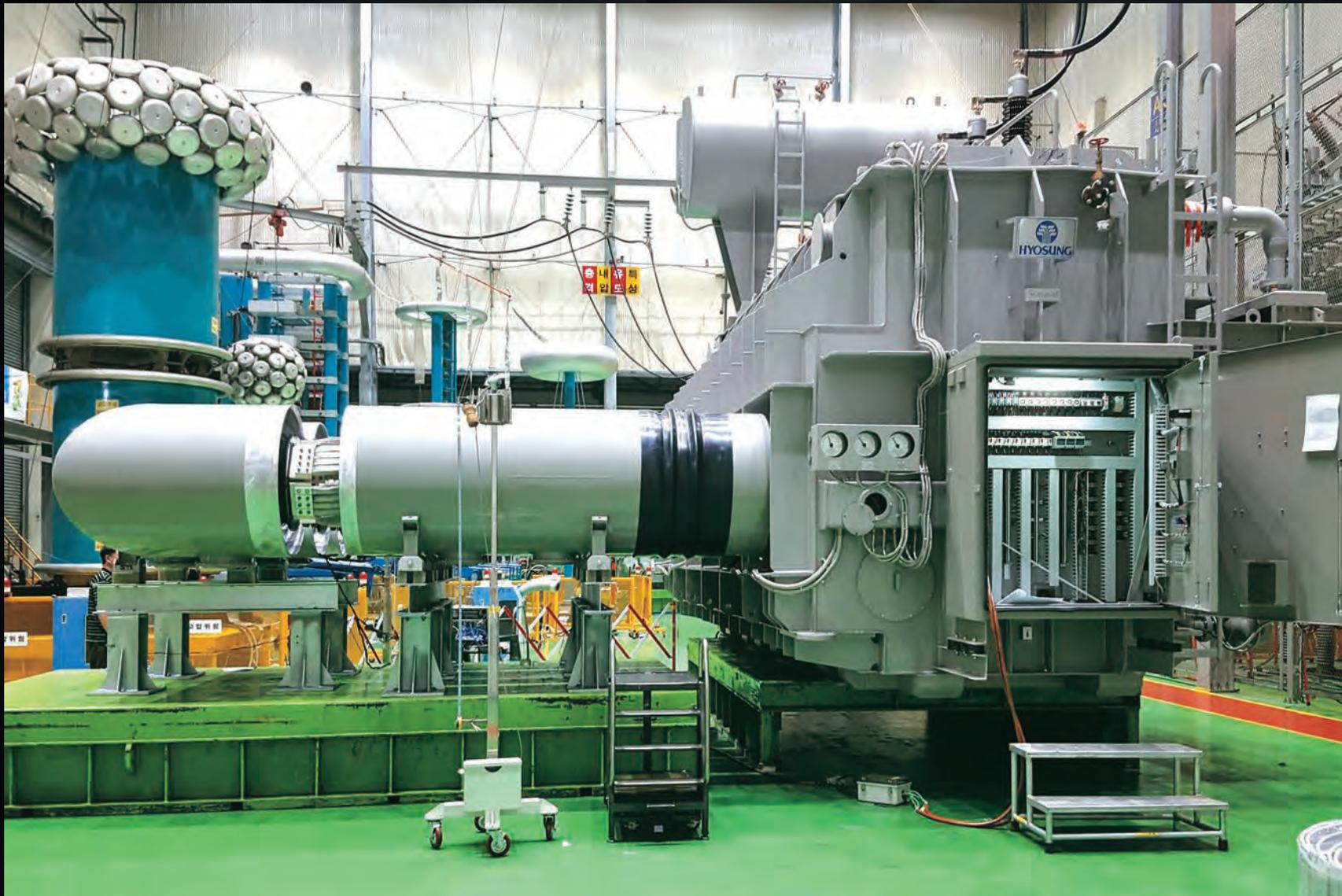
A 130-tonne converter/transformer is tested at the Korean firm Hyosung. It is one of 12 that will be delivered to ITER to transform current for the central solenoid magnet system.
