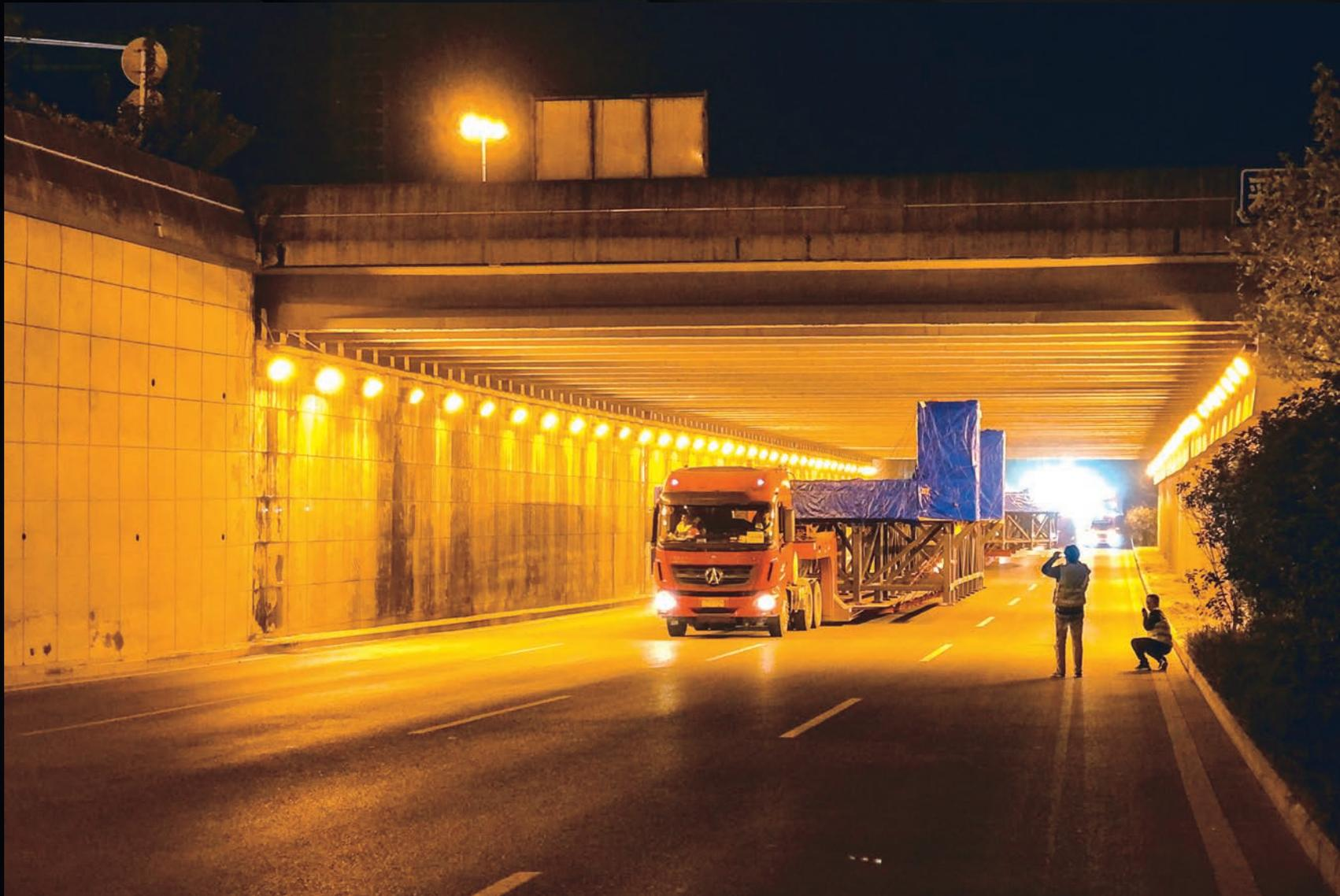
Several large semi-circular components have been delivered for the magnet feeder system that will transport cryogenics and electrical power to the bottom correction coil magnets. The feeder sections seen travelling here will be installed inside the cryostat base.
