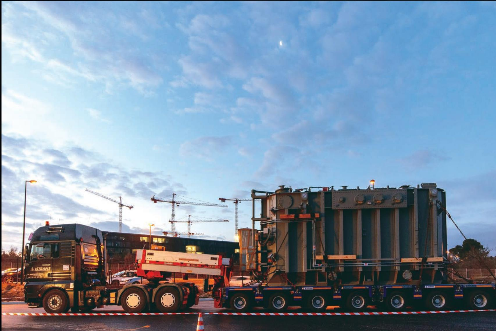
A 90-tonne electrical transformer procured by the United States is the first component to be transported along the ITER itinerary. At least 250 "highly exceptional loads" are expected during the construction and assembly phases of ITER.
