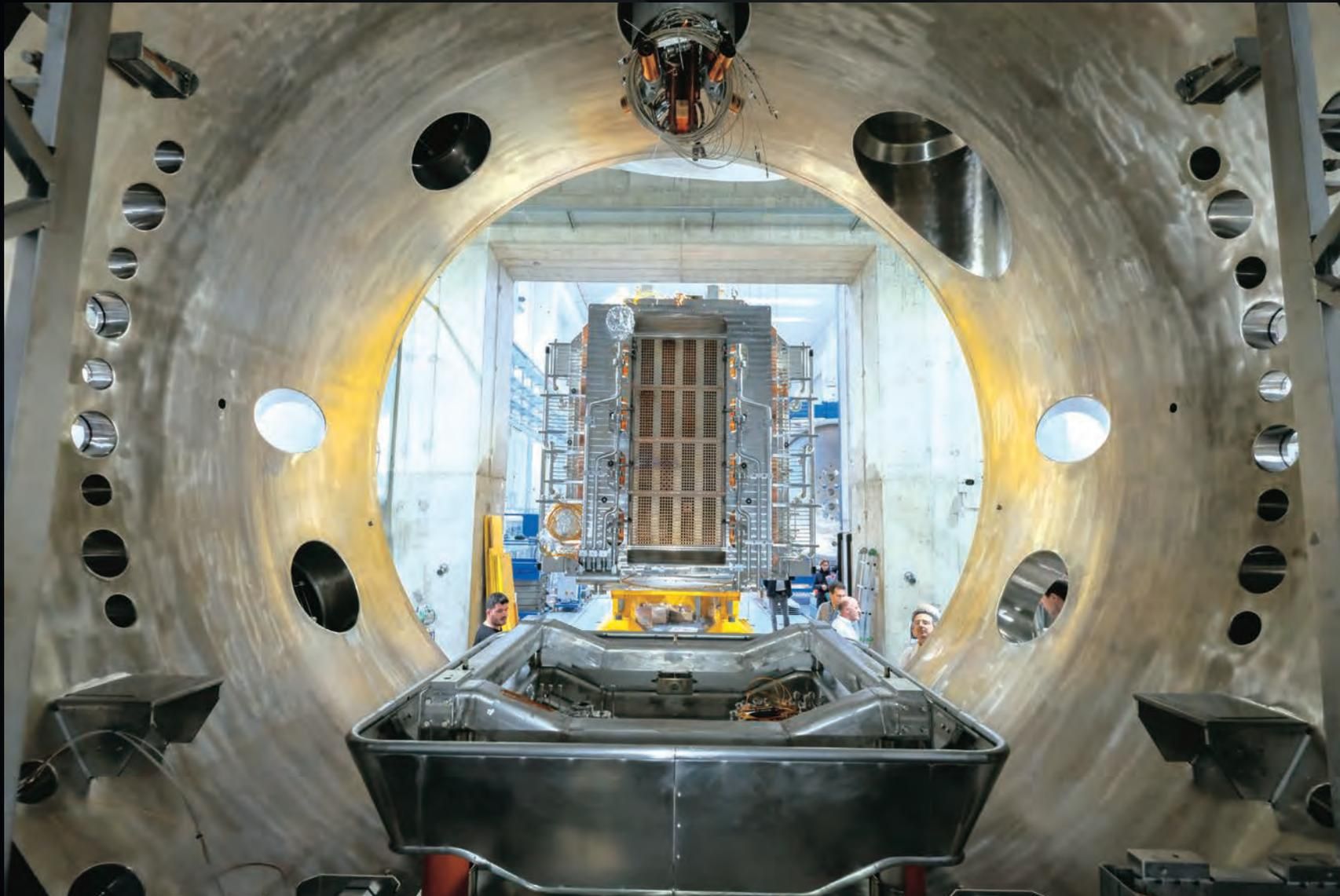
After a two-year shutdown for upgrades, the SPIDER testbed at the ITER Neutral Beam Test Facility in Padua, Italy, is preparing for commissioning and operation. SPIDER is a full-size negative ion source that is designed to demonstrate all the critical aspects of the ion sources for ITER's heating and diagnostic neutral beam injectors.
