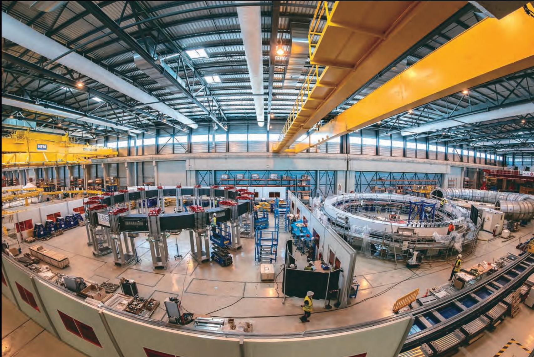
From left to right: two poloidal field coils and a cryogenic chamber for cold testing are visible in this photo taken in July in the European manufacturing facility on site. Cold testing a completed coil is part of a test protocol that allows operators to simulate the thermal stresses and the work conditions that will be experienced by the magnet coils during operation.
