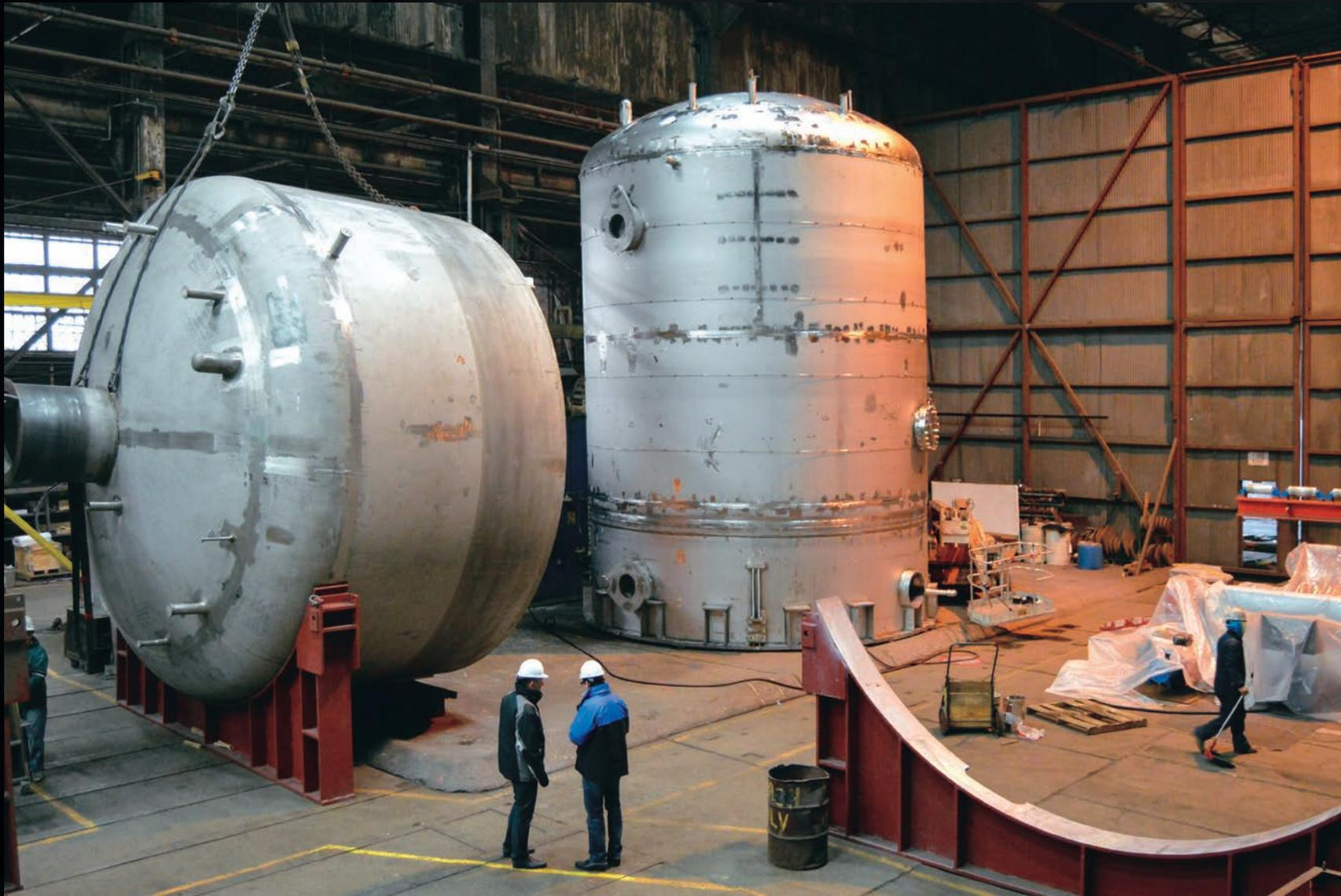
Drain tanks for the tokamak cooling water system are in fabrication at Joseph Oat Corporation in Camden, New Jersey.
