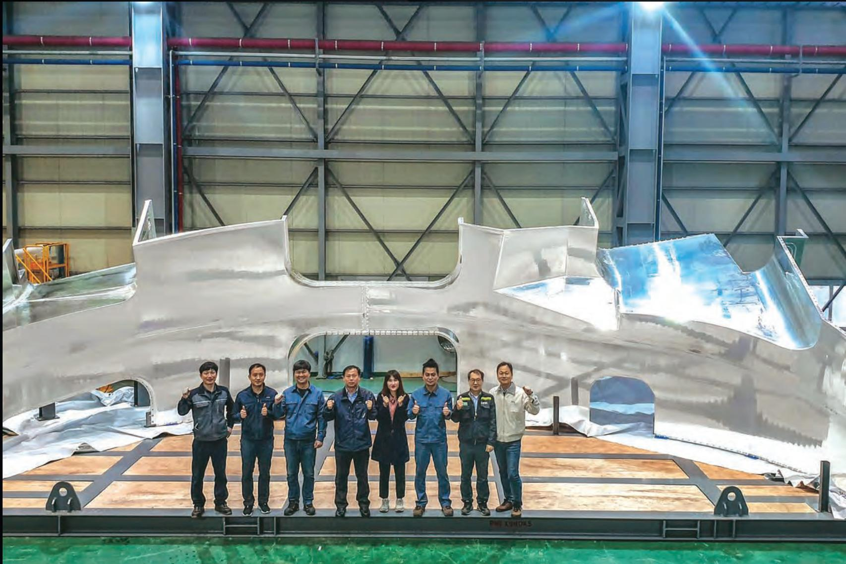
Six years after the start of fabrication, Korean contractor SFA completes the final 40° sector of the vacuum vessel thermal shield. The stainless-steel panels will be mounted on vacuum vessel sectors before they are lowered into the assembly pit.
