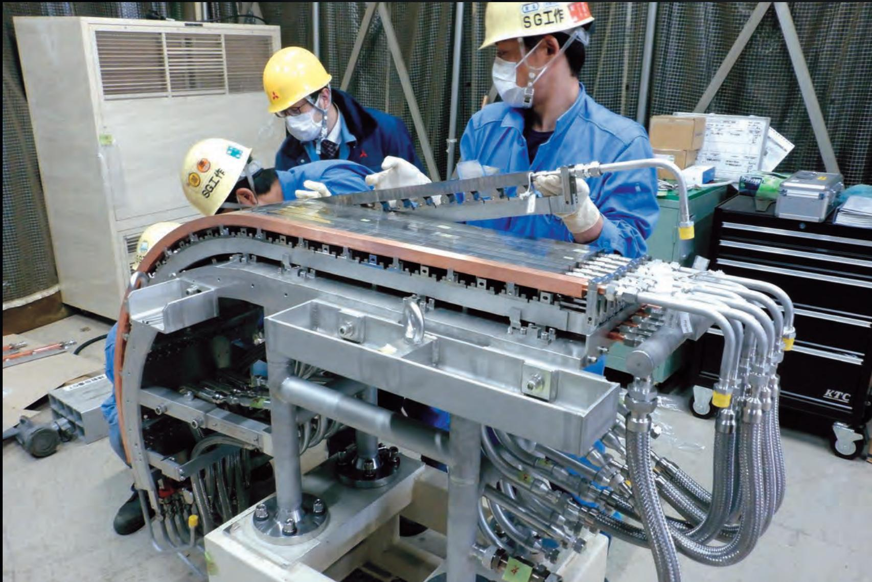
Japan is in the last phase of qualifying the divertor outer target, which will be exposed to the highest heat load of the ITER machine (on the order of 20 MW/m<sup>2</sup>). Here, plasma-facing elements are mounted on a test assembly for high-heat-flux testing.
