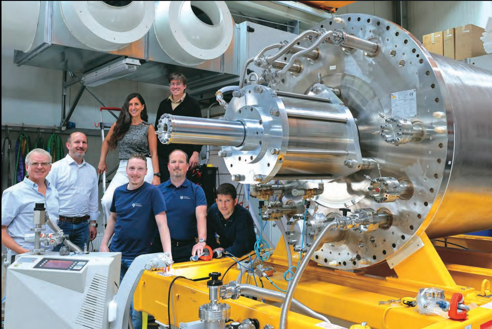
The first cryopump has passed factory acceptance tests at Research Instruments, Germany. ITER will rely on six torus cryopumps to maintain ultra-high vacuum inside the ITER vacuum vessel during operation and to create low density—about one million times lower than the density of air.
