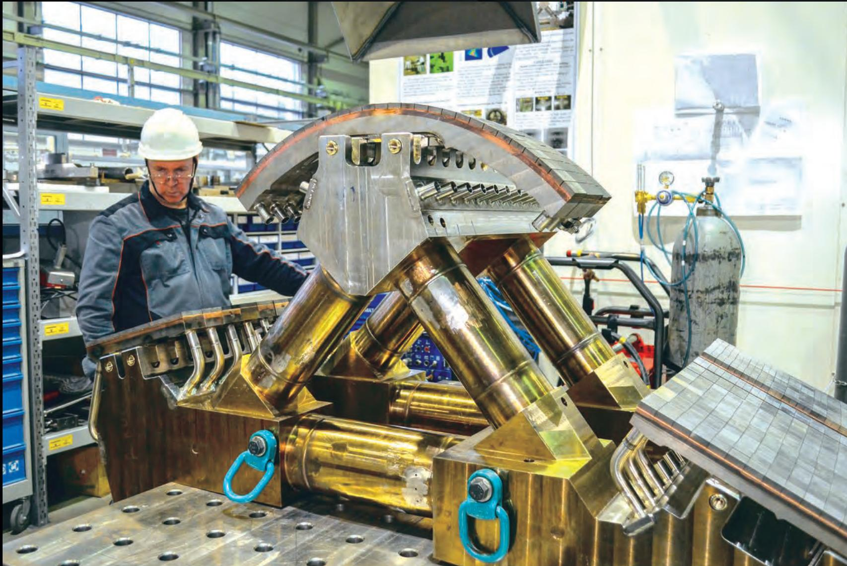
The Russian Federation has completed the first full-scale prototype of the divertor dome. One of three divertor targets designed to sustain the top heat flux of the ITER machine (10 to 20 MW/m<sup>2</sup>), a dome component will be mounted on each of the 54 divertor cassettes.
