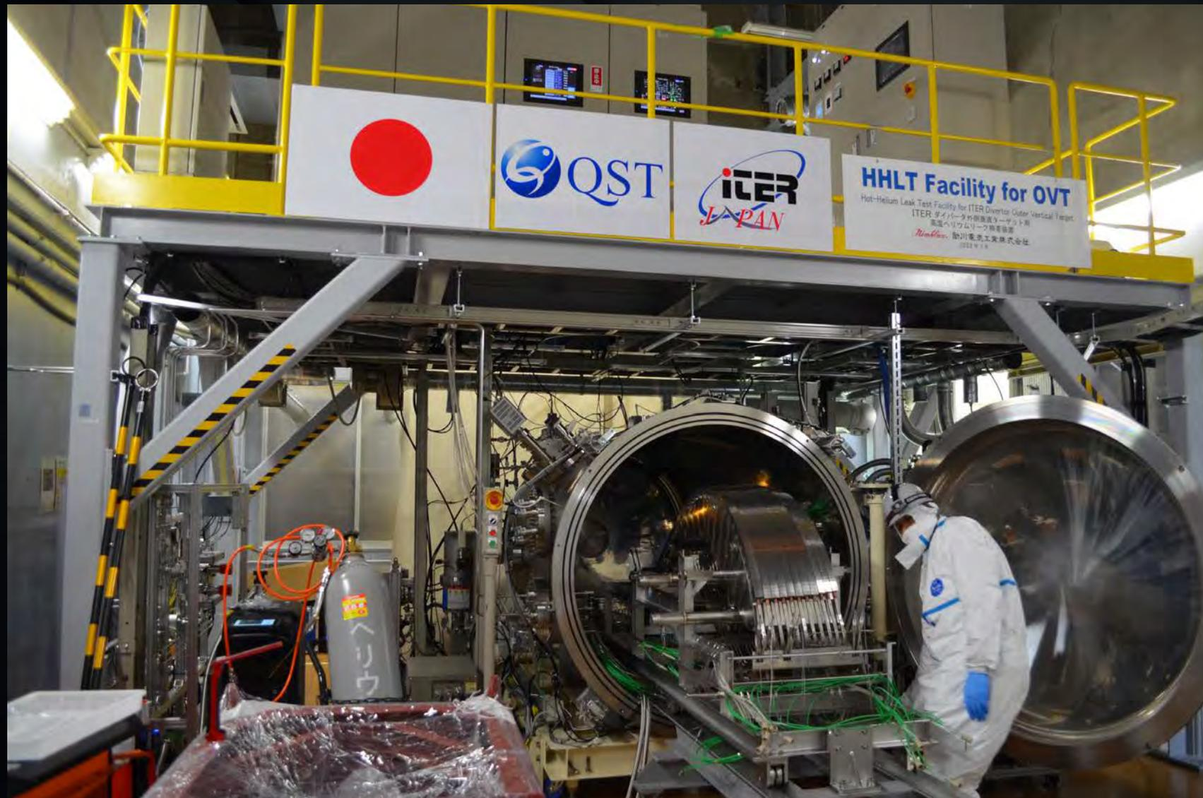
Prototype of the Divertor Outer Vertical Target (OVT) manufactured by Mitsubishi Heavy Industries was installed to the vacuum vessel of the Hot Helium Leak Test facility in JADA Naka-site. Stringent leak tightness of OVT prototype at room temperature and 250 oC was demonstrated.
