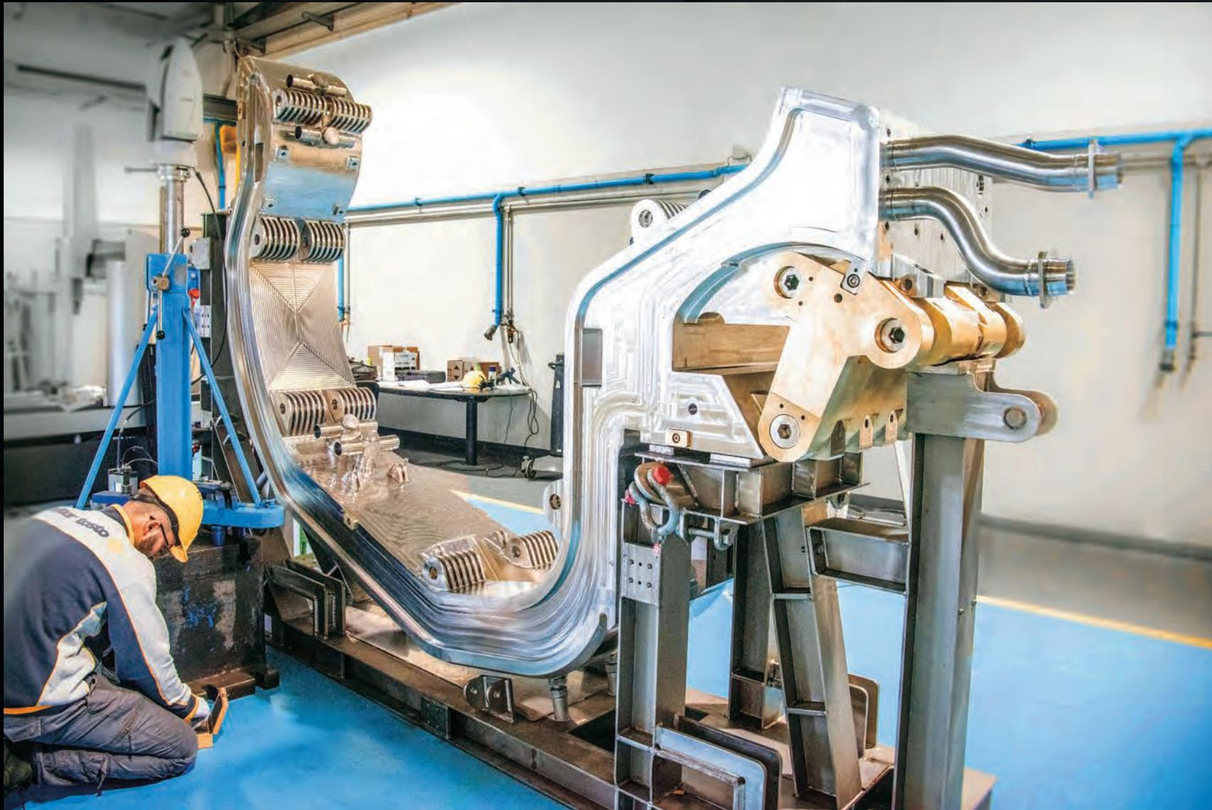
Divertor cassette bodies are the "chassis" of the divertor assemblies – eight-tonne structures that will support plasma-facing targets, diagnostics, operational instrumentation and cooling. Pictured is a real-size prototype manufactured in Italy by Water Tosto.
