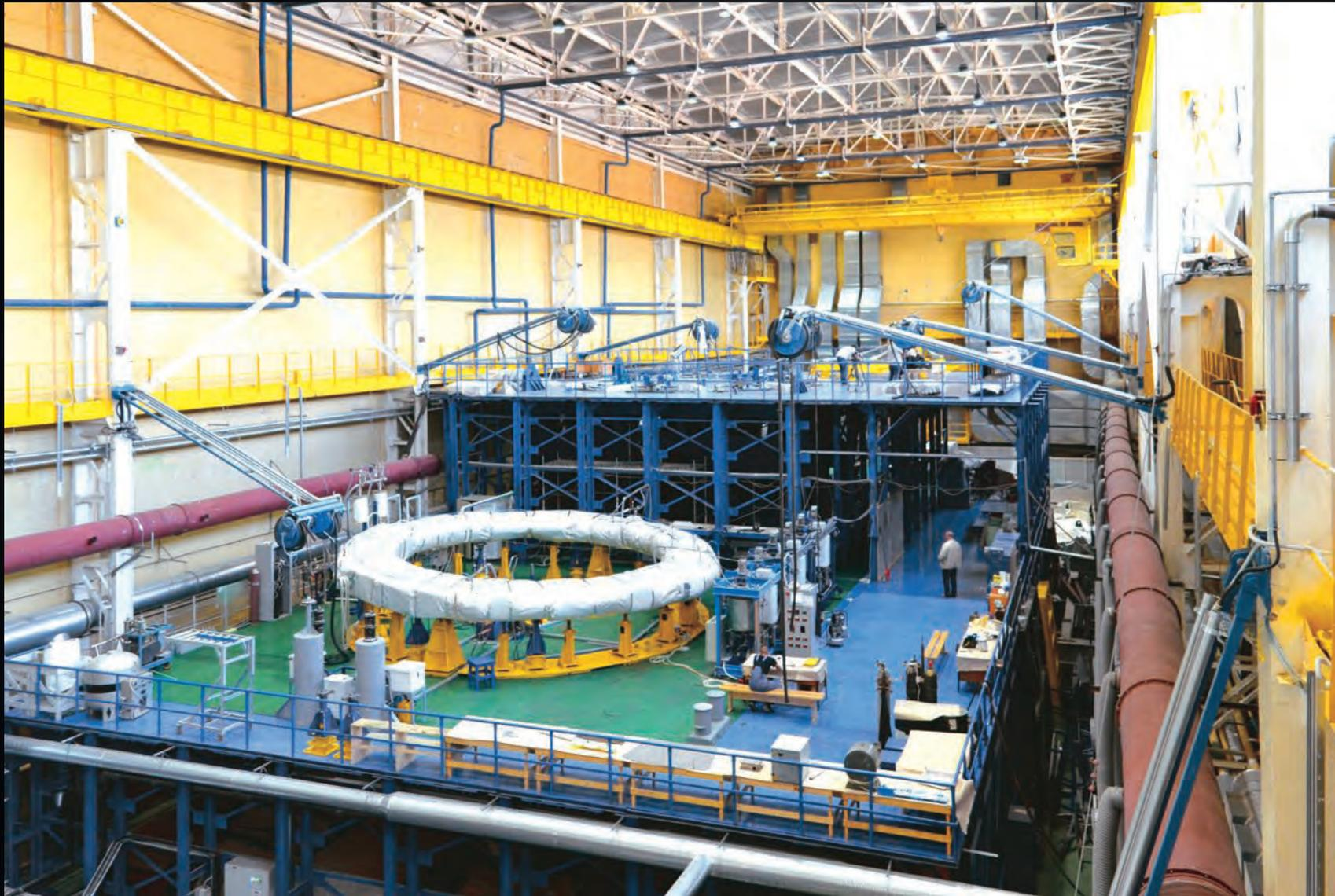
In St. Petersburg, Russia, specialists of the Efremov Institute and the Srednenevsky shipyard have completed the first poloidal field double pancake winding. Eight double pancakes will be stacked to form poloidal field coil #1, the smallest of ITER's ring-shaped magnets.
