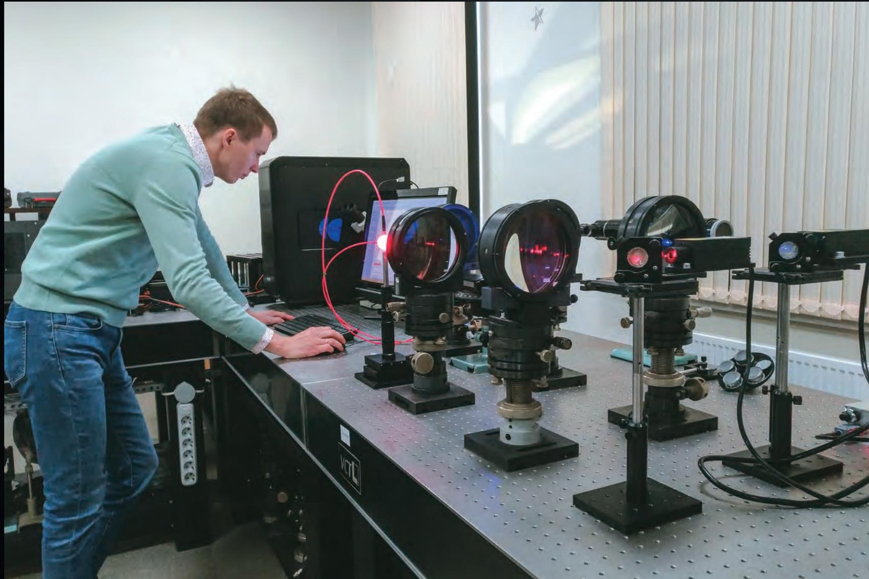
A spectroscopic laboratory has been created in Moscow to support the development of the optical diagnostic systems, which are used to measure temperature and density profiles at the core or the edge of the ITER plasma.
