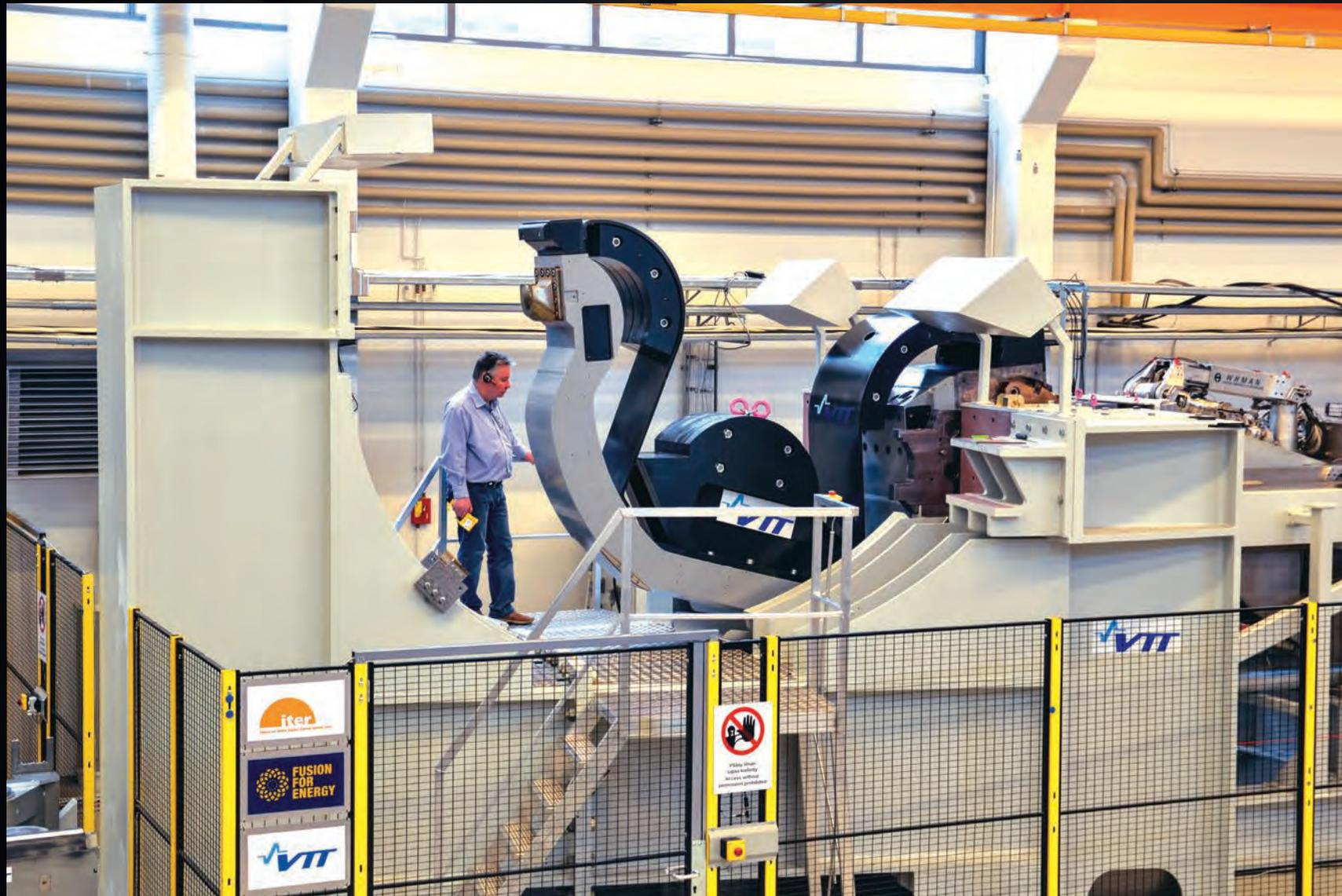
Europe is responsible for procuring the remote handling systems for the ITER divertor. Pictured: the final demonstration of cassette remote handling is successfully performed at the DTP2 Divertor Test Platform facility in Tampere, Finland.
