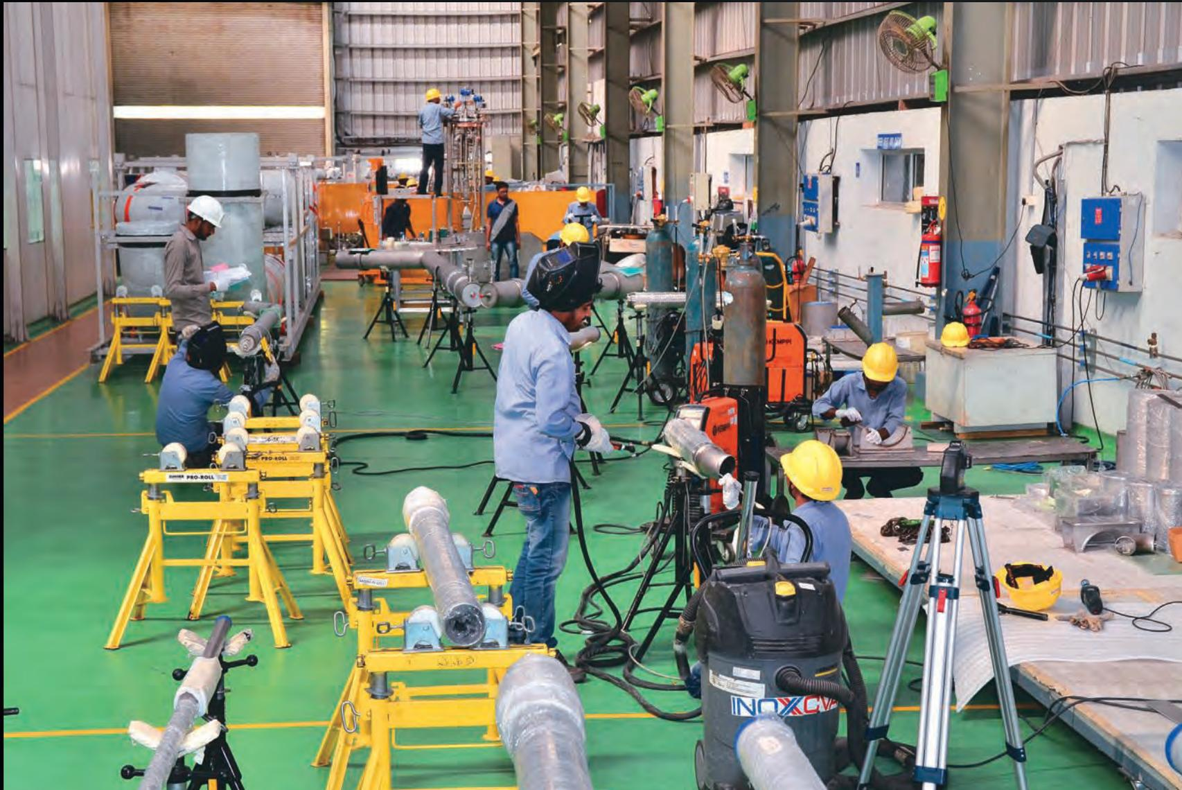
Procurement for the ITER cryolines—the highly sophisticated multi-process pipes that transport cooling fluids—is shared by France's Air Liquide and India's INOXVA (pictured here). ITER will have approximately 5 kilometres of cryolines ranging from 25 to 1000 millimetres in diameter.
