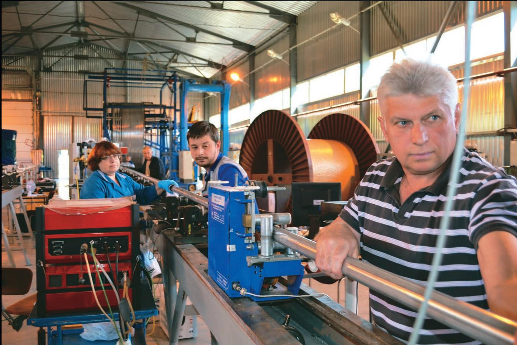
In June, specialists from the Cable Institute (JSC VNIKIP) jacket and compact the last production length of Russian toroidal field conductor at the Institute of High Energy Physics in Protvino, Russia. This milestone marks the end of a five-year campaign to manufacture 28 production lengths, amounting to more than 120 tonnes of material.
