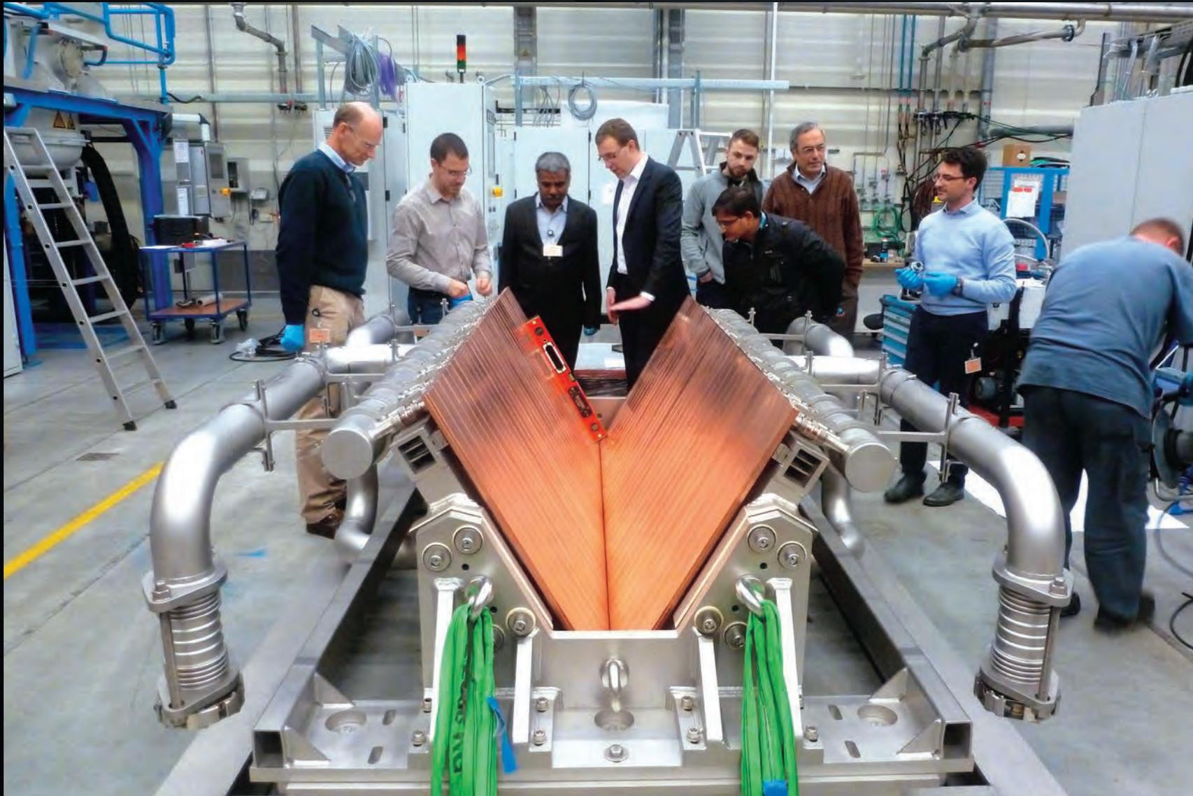
In December 2014, India celebrates its first delivery for the ITER Project—a beam dump for the full-scale ion source test bed at the ITER Neutral Beam Test Facility in Padua, Italy.
