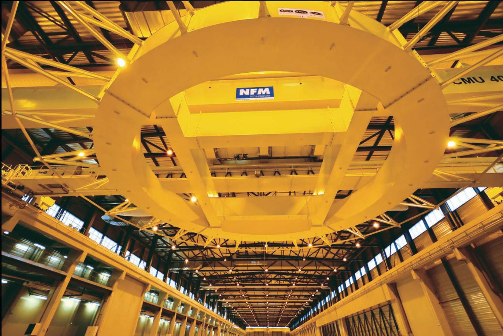
Inside Europe's on-site Poloidal Field Coils Winding Facility, a large sun-like spreader beam has been installed for the delicate transport of double pancake windings from station to station.
