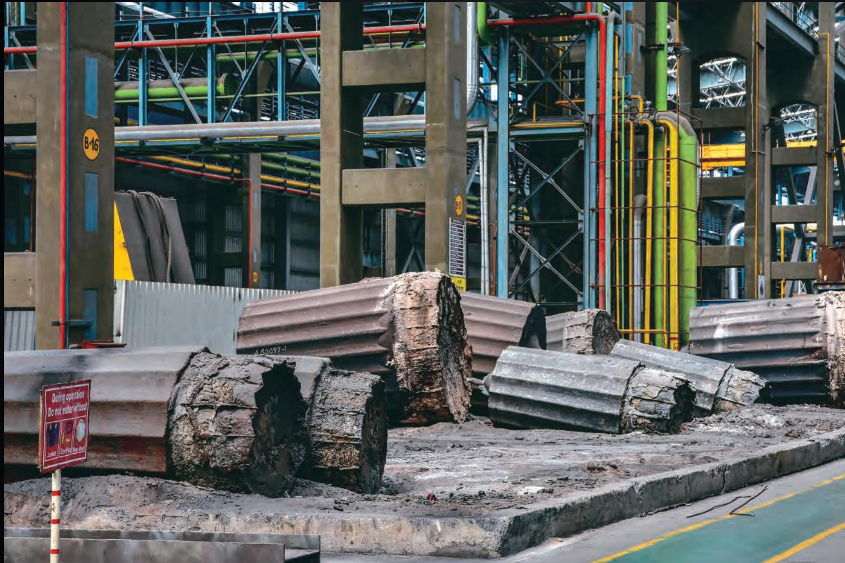
Doric or Ionic? Neither. What looks like broken columns from a Greek temple are in fact steel ingots for the ITER cryostat, cooling on a bed of black sand inside the Larsen & Toubro Ltd foundry in Hazira, India.
