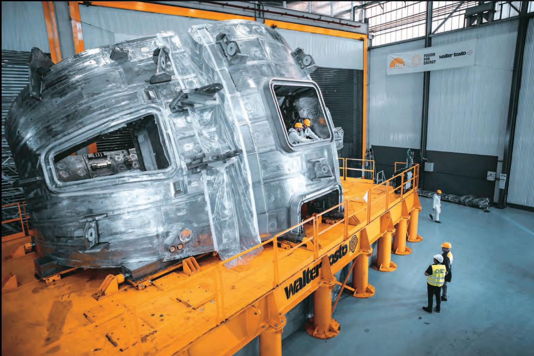
Each vacuum vessel sector is assembled from four smaller segments. In this photo of Europe's sector 4, we can see two segments coming together.
