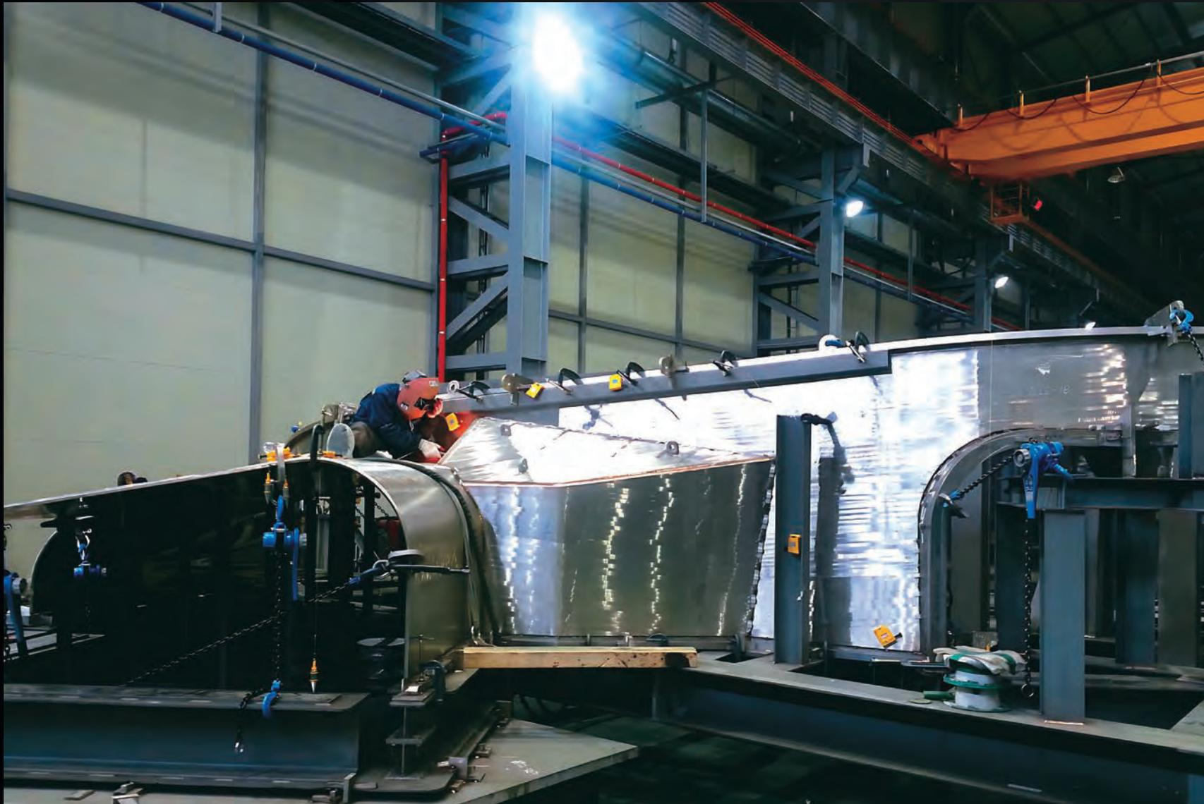
A thin barrier of stainless steel (10-20 mm), actively cooled and covered with a low-emissivity coating of silver, will protect the magnet coils from thermal radiation. At SFA Engineering in Changwon, Korea, welding is underway on an outboard sector of the vacuum vessel thermal shield.
