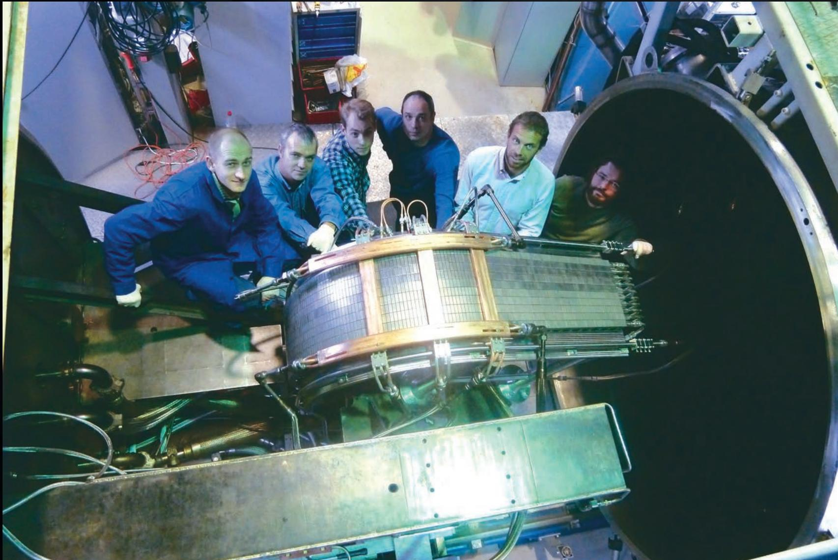
This plasma-facing component of the ITER divertor – a full-scale prototype of the inner vertical target manufactured by Ansaldo Nucleare and ENEA in Italy – is about to be tested under high heat flux at the Divertor Test Facility in Russia.
