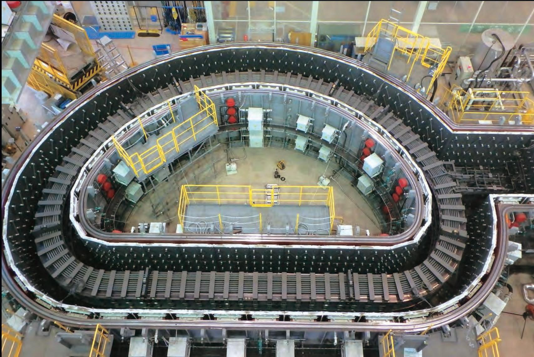
Toroidal field coil windings must be heat treated at 650 °C for 100 hours to react tin and niobium and form the superconducting compound Nb<sub>3</sub>Sn. In this furnace at Mitsubishi Heavy Industry's Futami factory, seven toroidal coil windings have been successfully heat treated.
