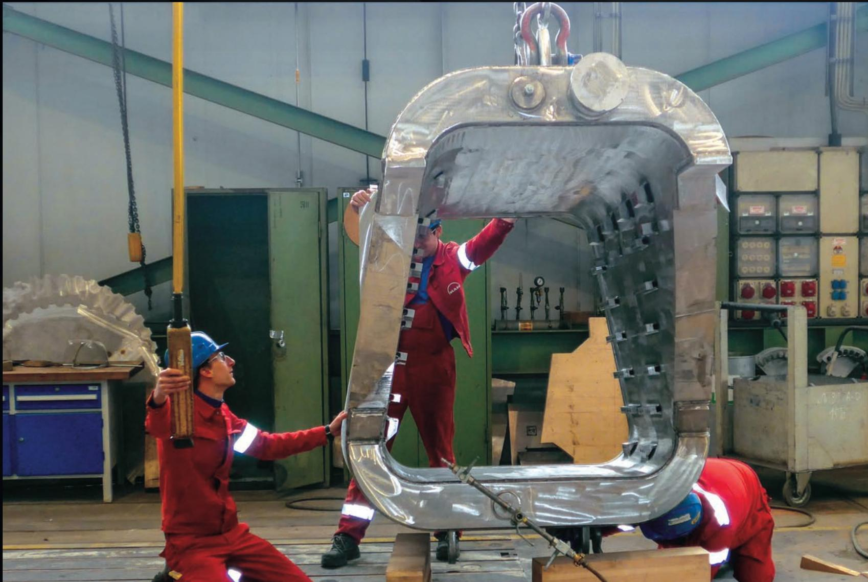
Extending out from each vacuum vessel port are port stub extensions that will be welded to the vacuum vessel sectors before the assembly of the main vessel in the pit. Russian contractors are producing extensions for the ITER upper ports in series.
