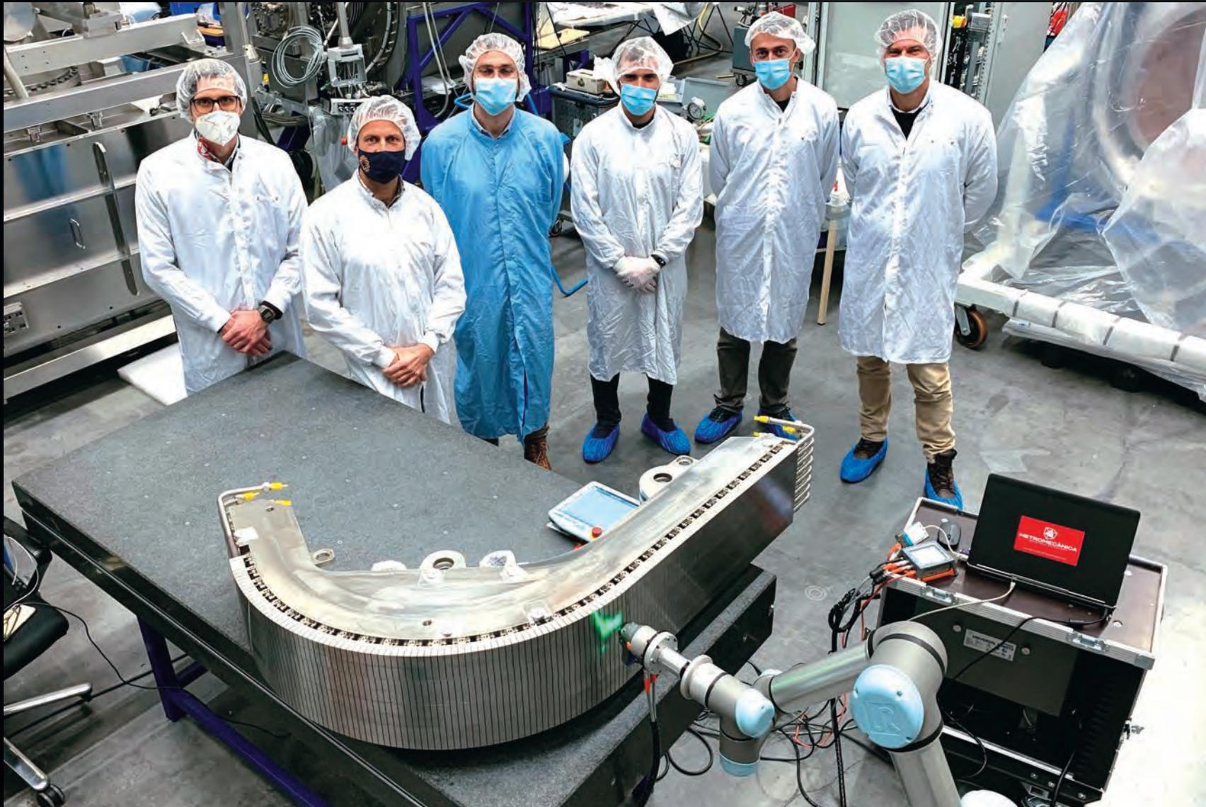
Representatives of Fusion for Energy, Research Instruments, and Metromecanica observe dimensional tests on a full-scale divertor inner vertical target prototype. The target's surface is made of small monoblocks in tungsten, which can withstand some of the highest heat loads of the ITER machine.
