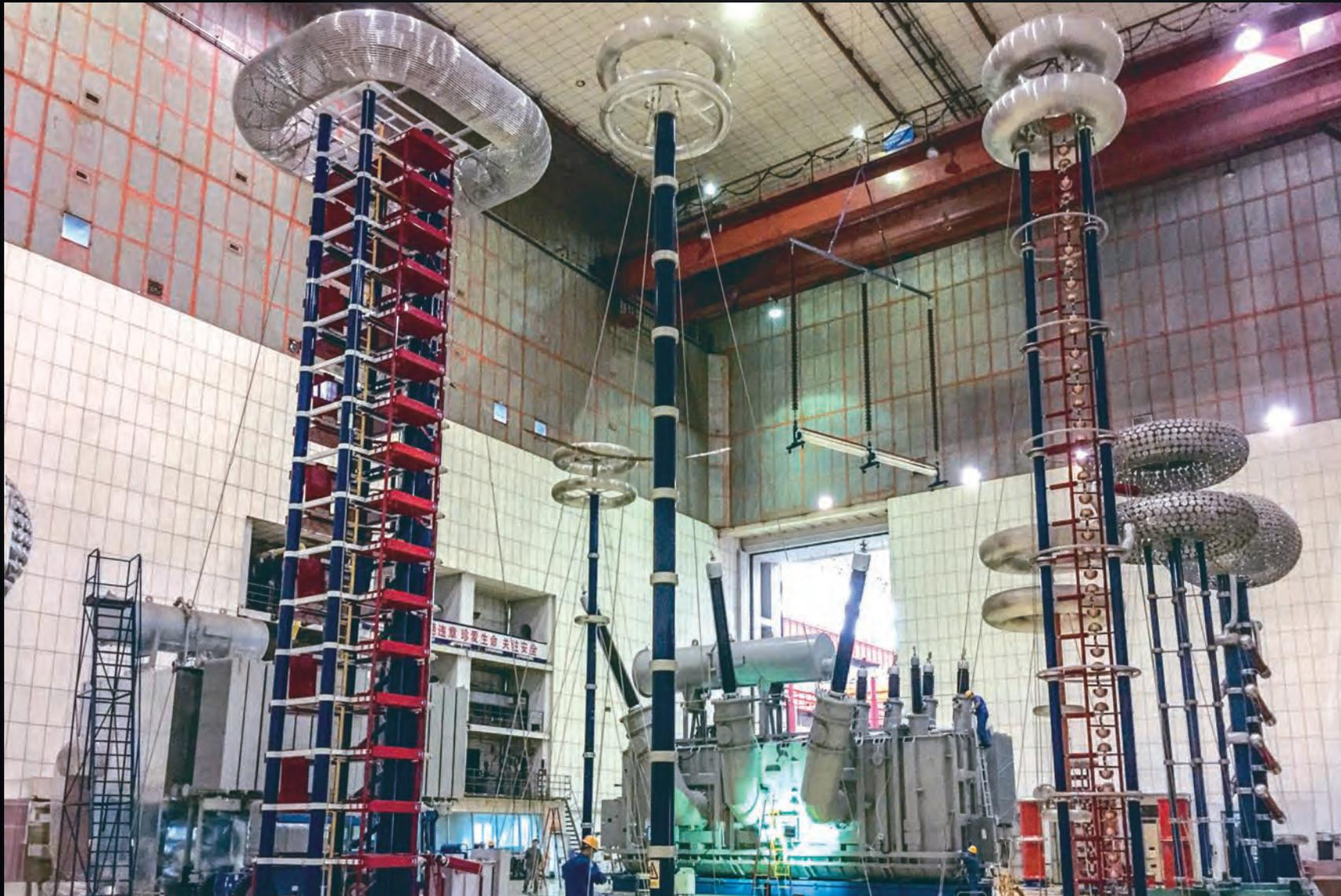
This 300 MVA step-down transformer is one of three that have successfully passed factory acceptance tests in China for ITER's pulsed power electrical network. The first transformer reaches ITER in 2016.
