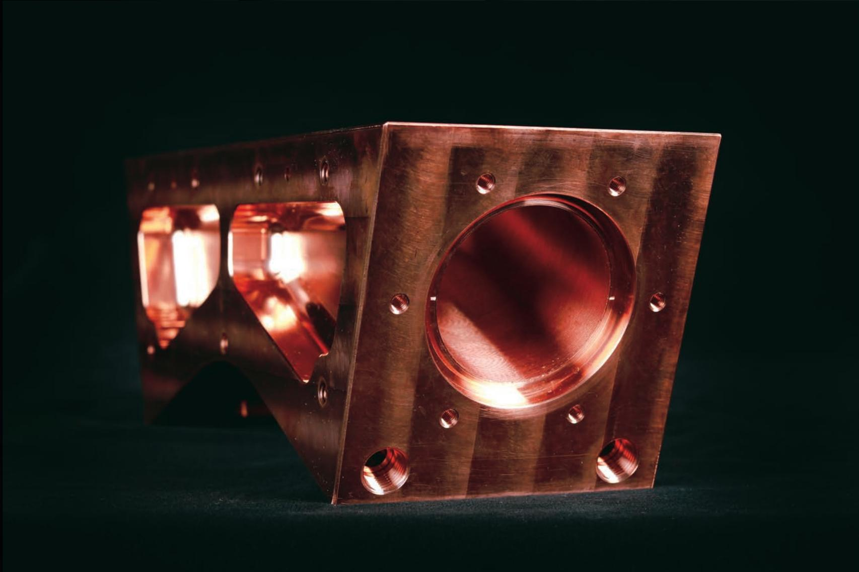
This "mitre bend" waveguide prototype is part of the electron cyclotron transmission lines that will route microwave beams from the Radio Frequency Building to the tokamak, where they will deliver 20 MW of heating power to the ITER plasma. Transmission line R&D, design and fabrication is under the responsibility of the US Domestic Agency.
