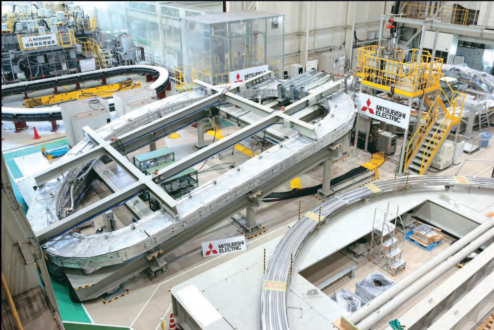
Double pancakes – the building blocks of the toroidal field winding packs – are produced in series at Mitsubishi Heavy Industries in Japan, passing through winding, insulation and finally impregnation stages.
