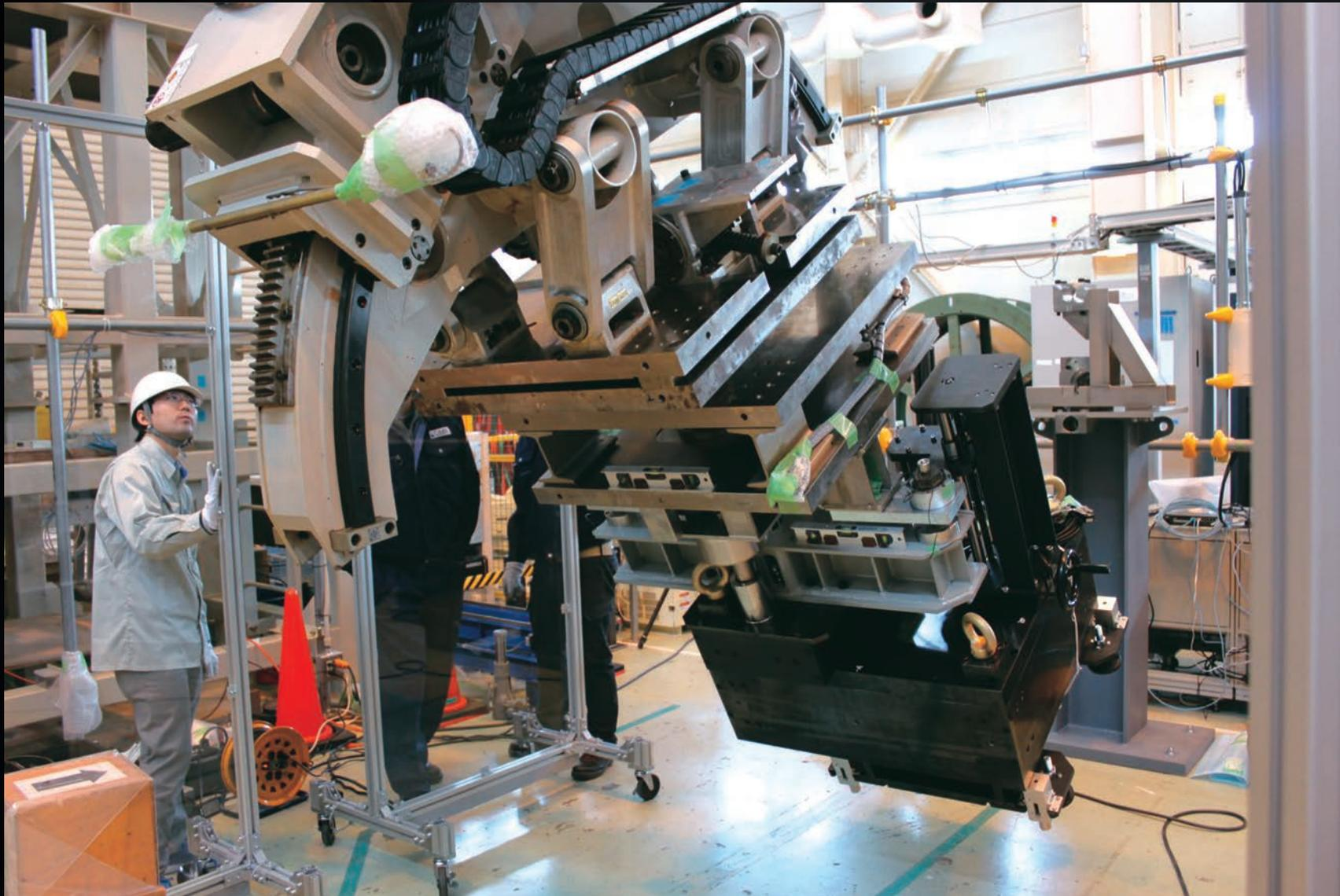
Although not as powerful as the Infinity Gauntlet of comic book fame, the robotic bolting tool that will be used to install ITER's in-vessel blanket modules is impressive. It will provide 10 kilonewton/metres (kNm) of torque to tighten the massive bolts of the blanket first wall panels.
