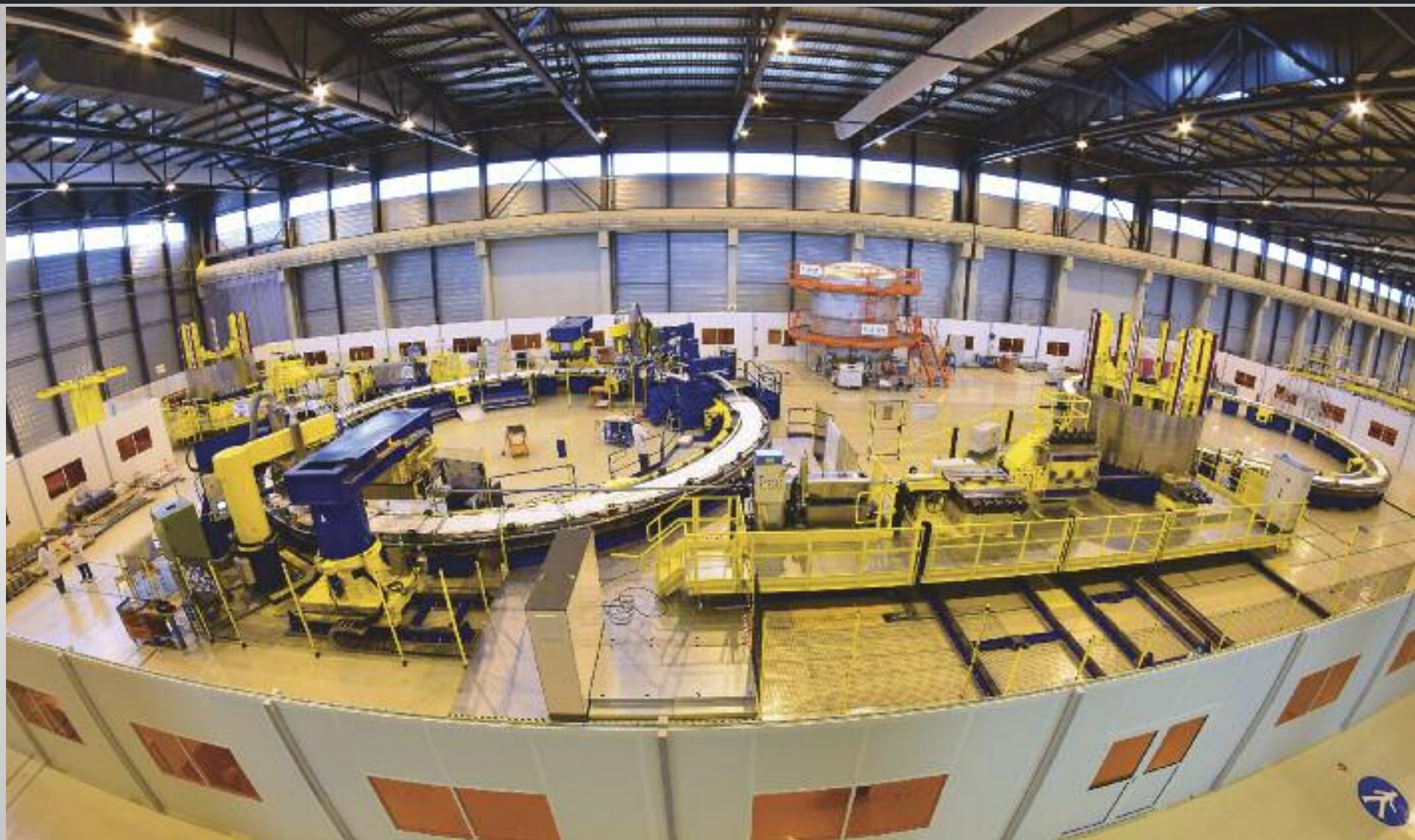
Four of ITER's six ring-shaped poloidal field coils will be manufactured by Europe in this on-site facility. In 2016, activities to qualify tooling and processes were successfully launched. November 2016
