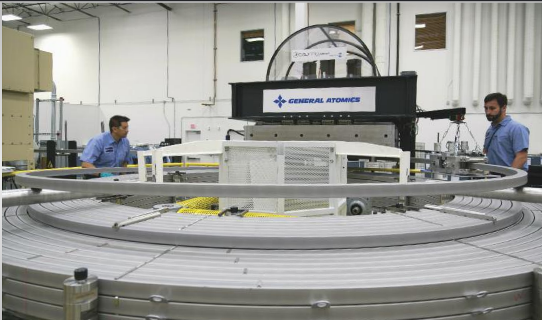
General Atomics technicians complete the winding of the first central solenoid module in April. Six modules – each made from approximately 6,000 metres of niobium-tin (Nb3Sn) superconductor supplied by Japan – will be stacked to form the 13-metre-tall central magnet.
