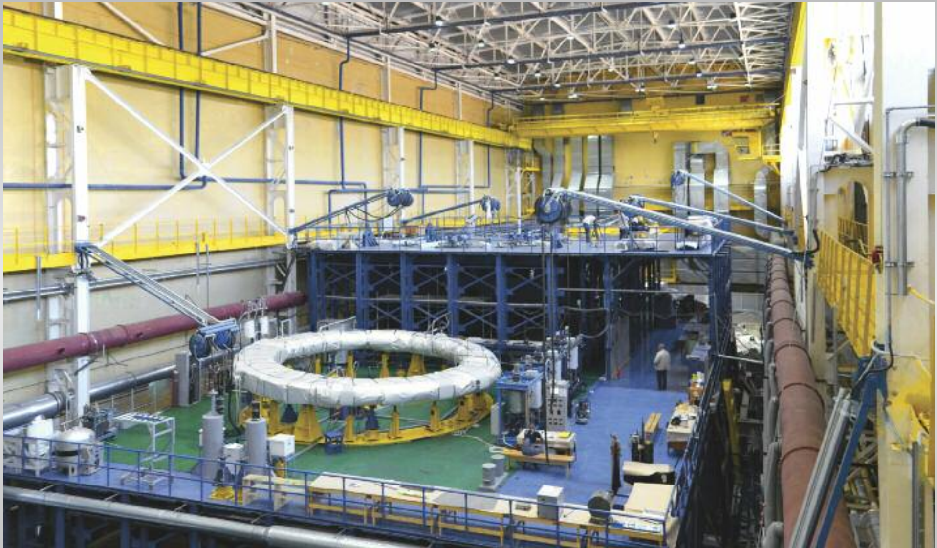
In St. Petersburg, specialists of the Efremov Institute and the Srednensky shipyard have completed the first poloidal field double pancake winding. Eight double pancakes will be stacked to form poloidal field coil 1, the smallest of ITER's ring-shaped magnets.
