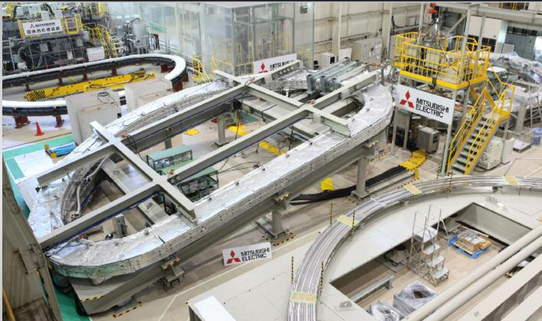
Double pancakes for the ITER TF coils are first insulated with glass and polyimide tape, then impregnated with cyanate-ester and epoxy resins to harden the assembly. Seven double pancakes for the first-of-series production – the building blocks of the toroidal field coils – have been insulated and impregnated at the Futami Plant of Mitsubishi Heavy Industries, Ltd./Mitsubishi Electric Co.
