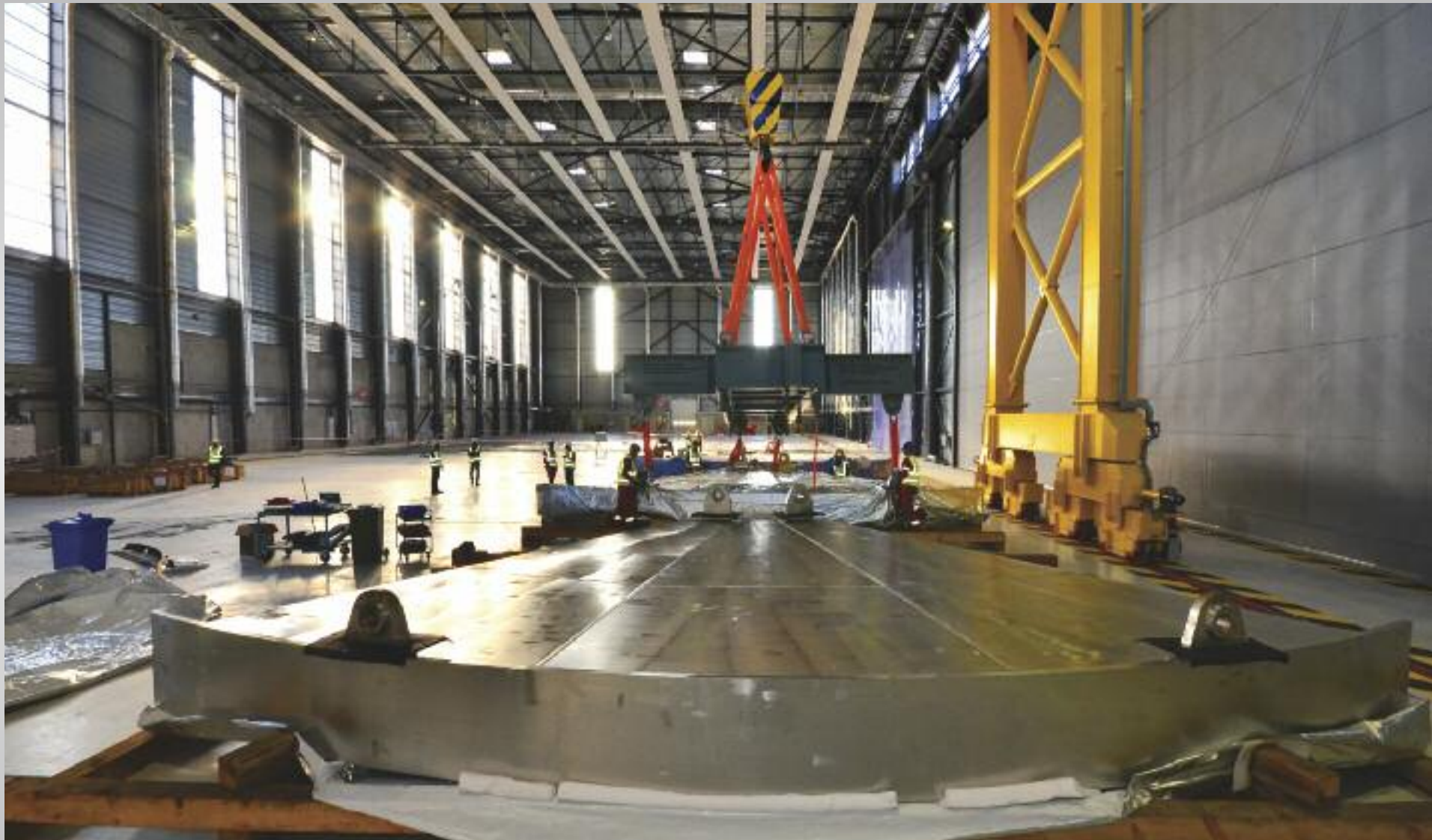
Advanced welding techniques such as automated, all-position narrow groove gas tungsten arc welding have been specially developed for the challenging assembly of 54 segments into the single largest component of the ITER machine. Pictured: two triangular segments for the cryostat base (tier 1) are stored in the Cryostat Workshop. December 2015
