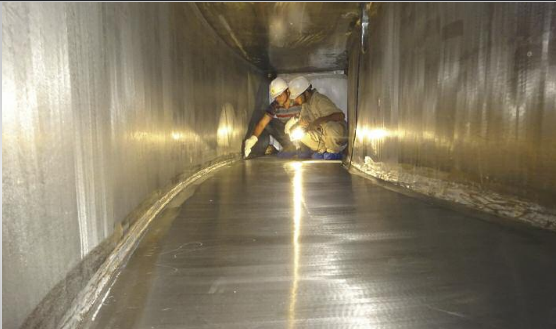
In the cryostat manufacturing facility in India, a segment of the pedestal ring (part of tier 2 of the base) is inspected before delivery to ITER. Responsible for the manufacturing design, fabrication and assembly of the 3,850-tonne ITER cryostat, India is shipping the cryostat to ITER in 54 segments for on-site assembly.
