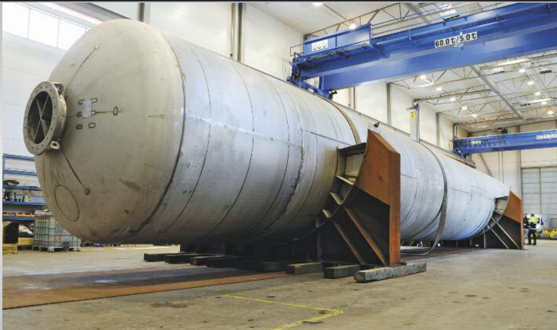
A 23-metre storage tank for liquid helium, part of Europe's contribution to ITER's liquid nitrogen plant and auxiliary systems, has successfully passed leak tests. The 190 m 3 stainless-steel tank will store liquid helium at -269 °C.
