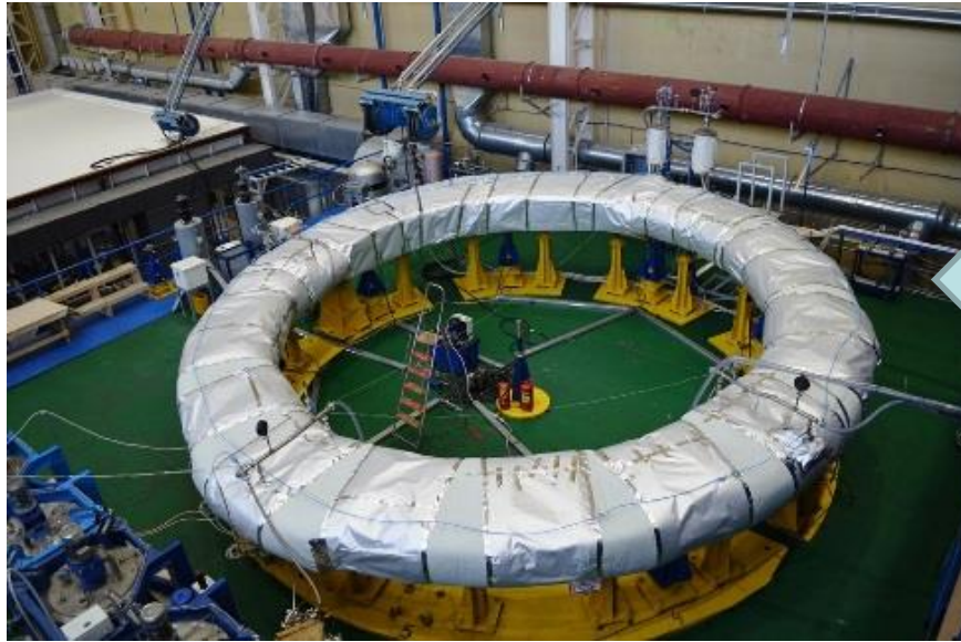
Vacuum impregnation (VPI) of 1st Double Pancake .
