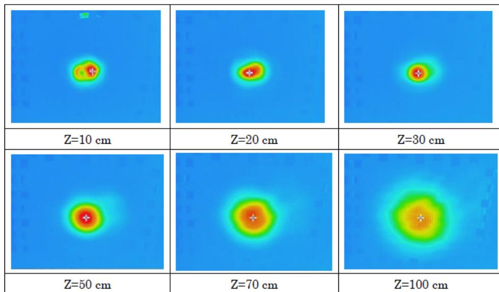
Output beam pattern at the output of MB7.
