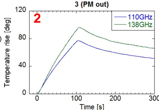
Maximum temperature close to the operational limit of Aluminum. ( $\sim 150^\circ\text{C}$ ) (initial temp.  $\sim 30^\circ\text{C}$ )
