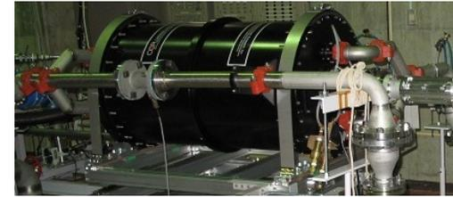
**30aP43** 1.5MW CW dummy load
