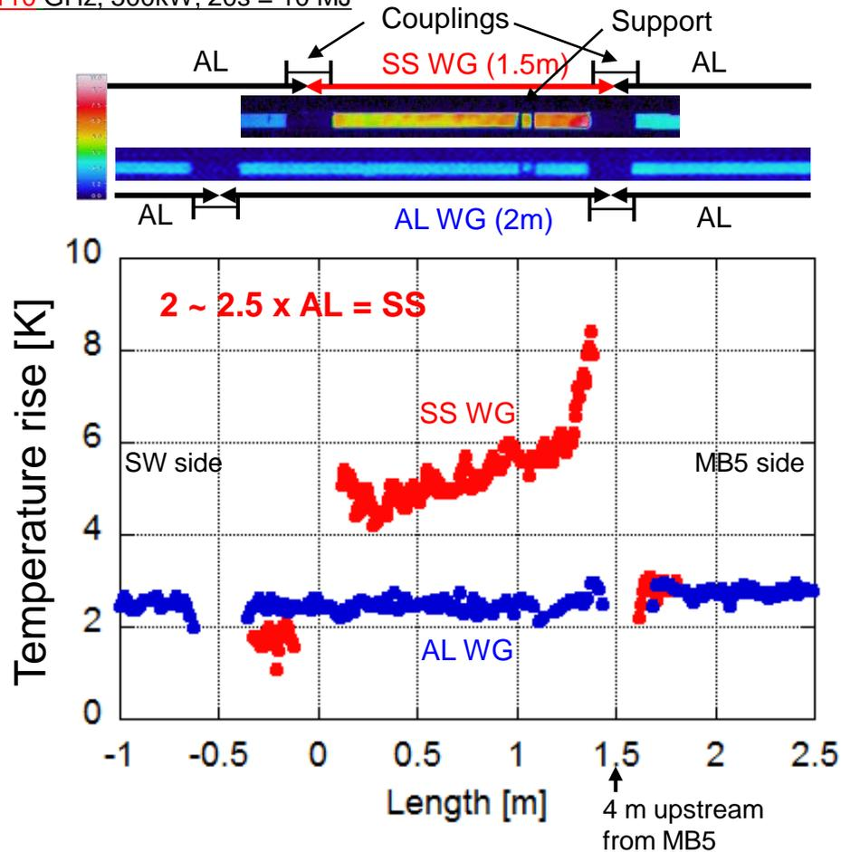
The waveguide used in air is made of aluminum alloy (AL) while the launcher, the stainless steel (SS) waveguide may be used in JT-60SA.
