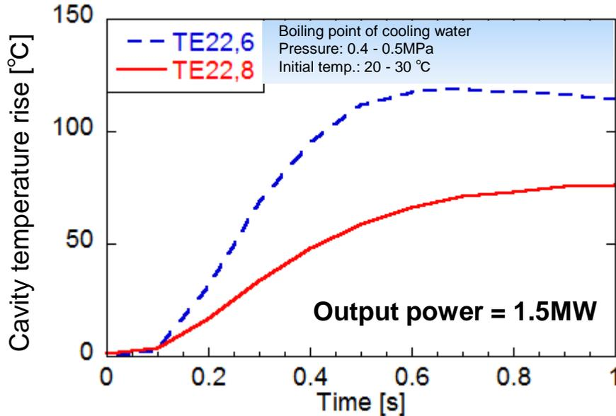
Measured by a thermocouple at the cooled surface of the cavity for both JT-60 (TE<sub>22,6</sub>) gyrotron and the JT-60SA gyrotron (TE<sub>22,8</sub>).
