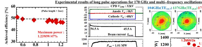
◆1.2MW power and ~ 50% efficiency have been demonstrated.
