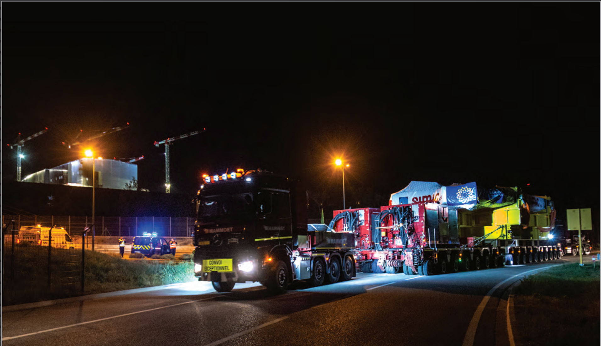
Europe's Fusion for Energy delivers the first D-shaped toroidal field coil of the ITER program (TF9) on 17 April 2020. Eighteen others are expected (including one spare) from Europe and Japan. April 2020
