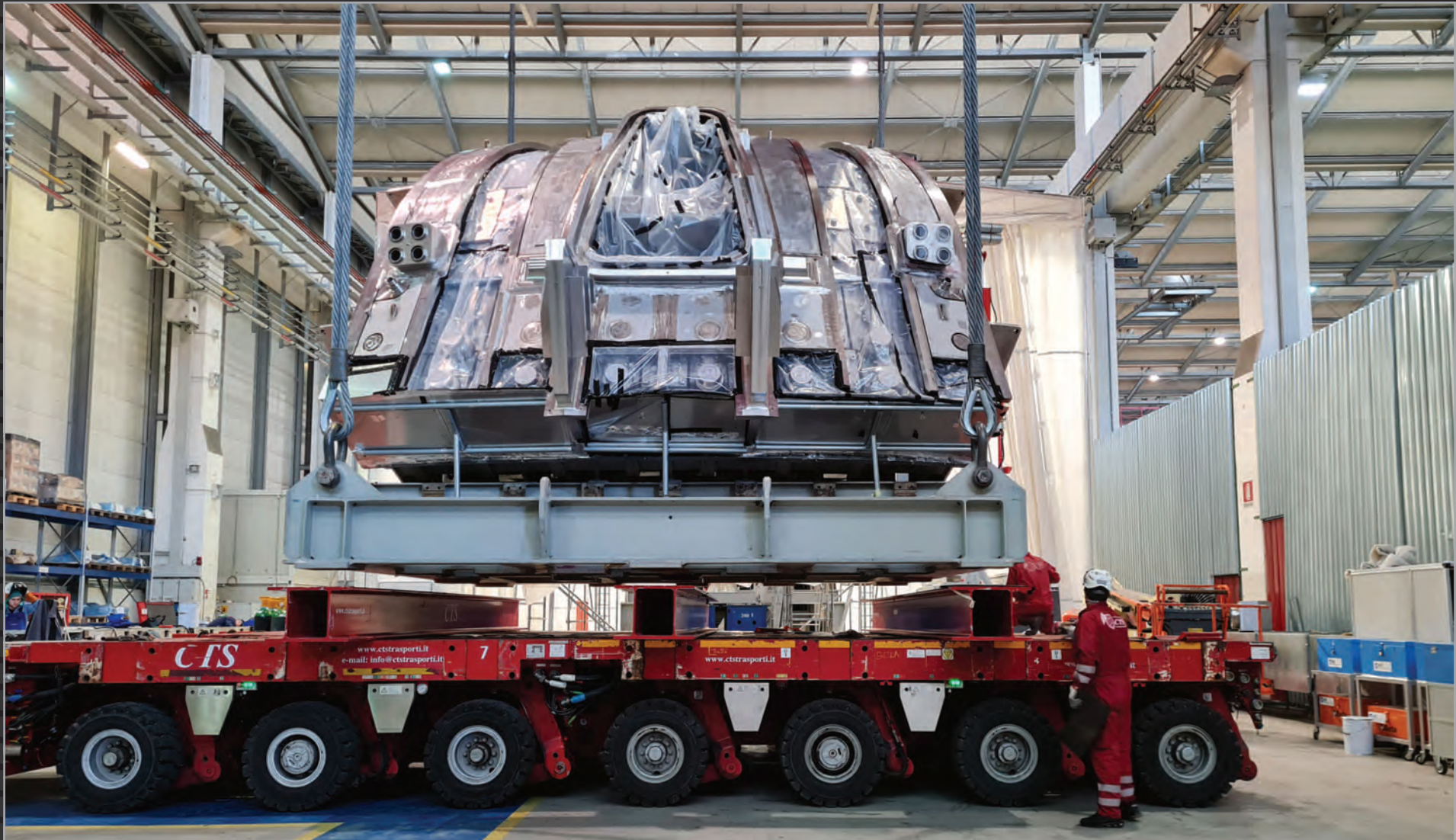
The European consortium AMW (Ansaldo Nucleare, Mangiarotti, Walter Tosto and subcontractors) is well advanced in the fabrication of five (of nine) sectors of the ITER vacuum vessel. Pictured is the shop floor at Mangiarotti, where one segment of sector #5 (the first expected at ITER) is nearing completion.
