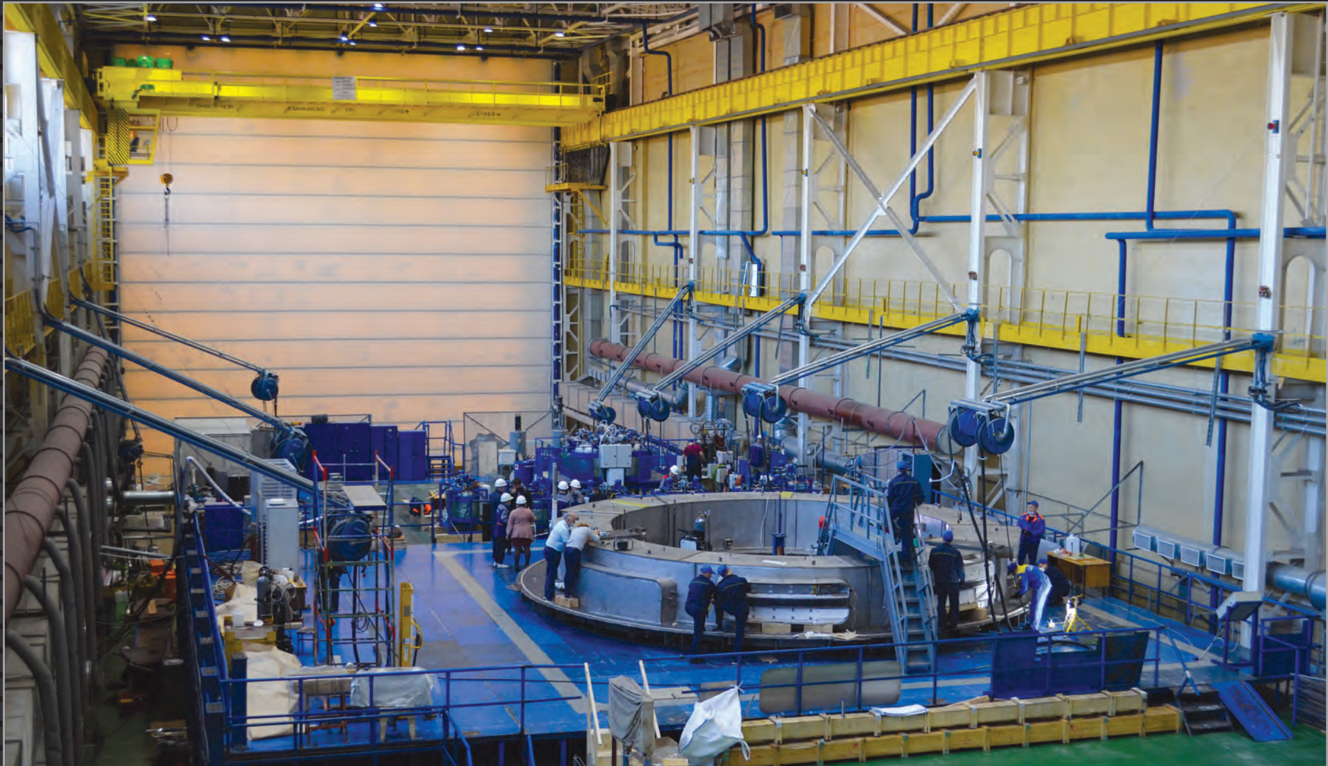
At the Sredne-Nevisky Shipyard near Saint Petersburg, ITER's smallest ring coil – PF1 – has successfully passed all winding tests; the next stage, impregnation, is imminent. The transport frame designed for this 200-tonne component is ready to enter service in late 2021.
