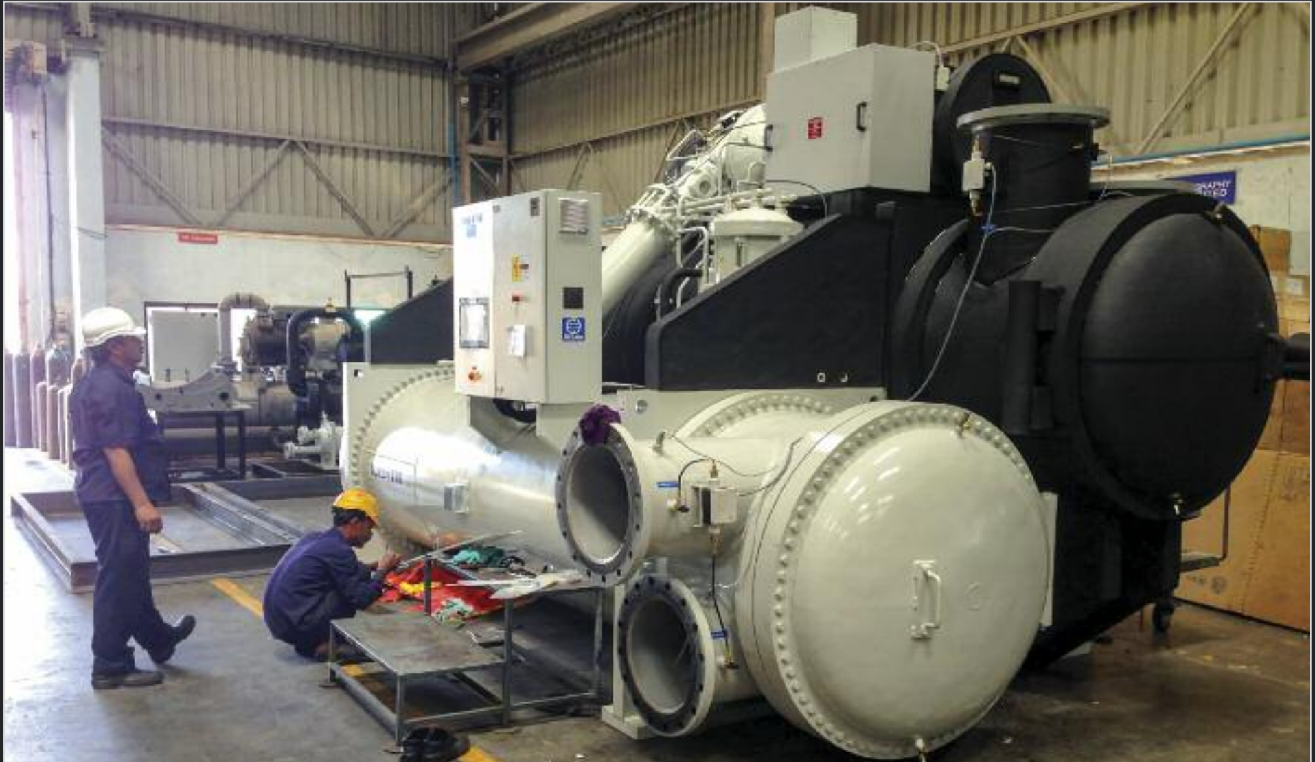
Work is underway in India to procure the components of ITER's component cooling water, chilled water and heat rejection systems. This large-capacity water-cooled chiller (one of eight required by the chilled water system) has successfully passed pre-shipment inspection at Kirloskar Chillers (Pune, Maharashtra).
