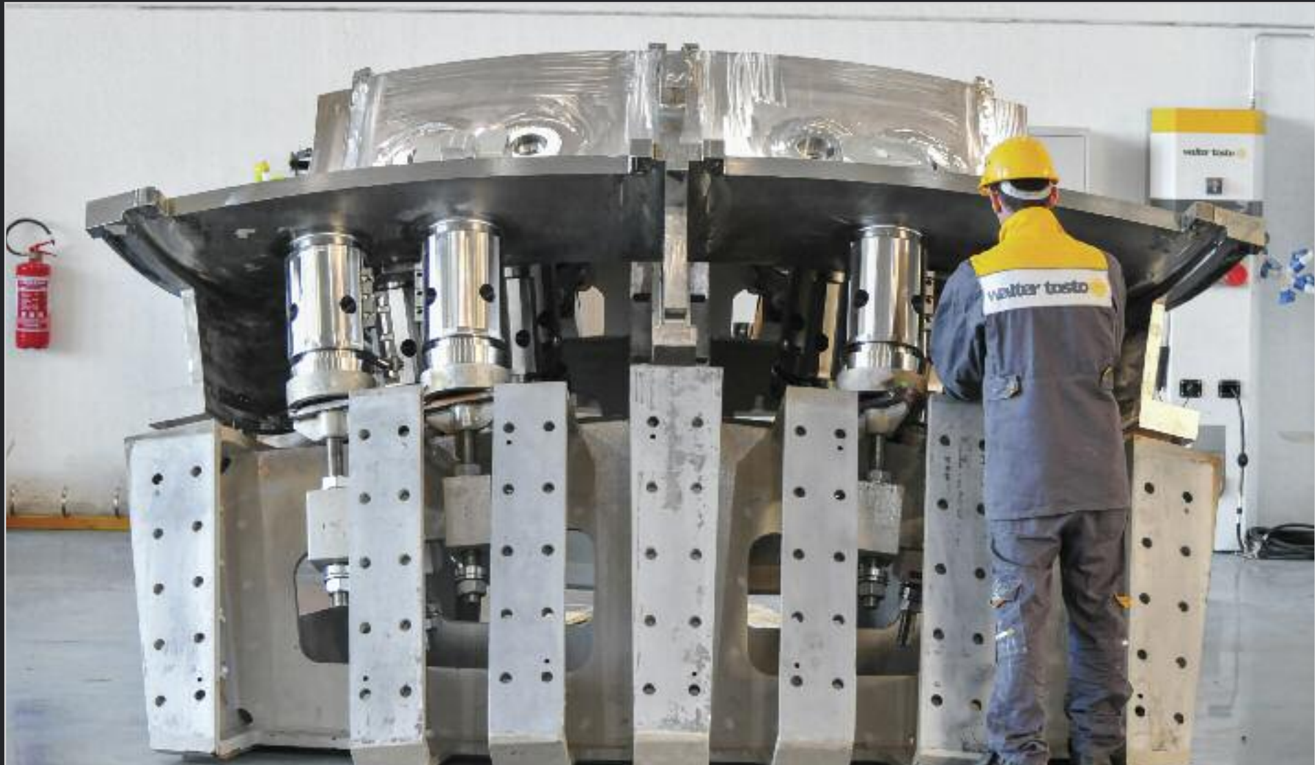
Five thousand tonnes of steel, dozens of "port" openings at three levels, interfaces with nearly every major system ... ITER's steel vacuum vessel is one of the largest-scale and most complex of the ITER "objects" to manufacture. In Europe, the AMW consortium is manufacturing five of the nine sectors (pictured: a sub-segment for sector #5).
