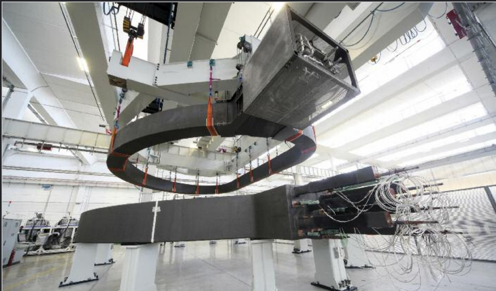
Eighteen toroidal field magnets – each made up of a 110-tonne winding pack and stainless steel coil case – will surround the vacuum vessel to confine the particles of the ITER plasma. The first 10 winding packs under European responsibility has left the ASG consortium in La Spezia, Italy.
