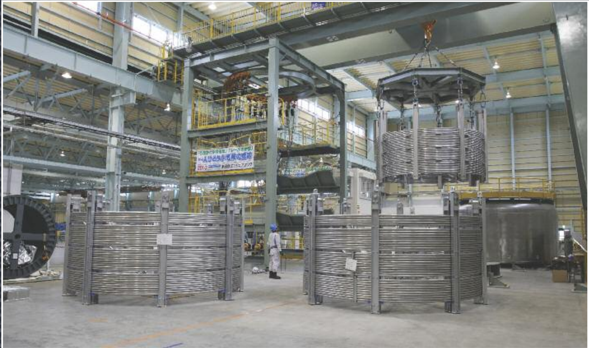
Upon the completion of jacketing, 760-metre-long toroidal field conductor unit lengths are spooled to facilitate transportation. In the image, three unit lengths are prepared for transport at the Wakamatsu factory, Nippon Steel & Sumikin Engineering.
