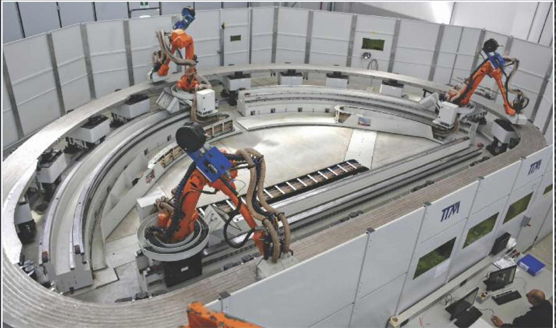
Toroidal field coil conductors will be shaped into layers called double pancakes, seven of which will constitute one toroidal field winding pack. Pictured, three laser welding robots work simultaneously on the double pancake cover plates.
