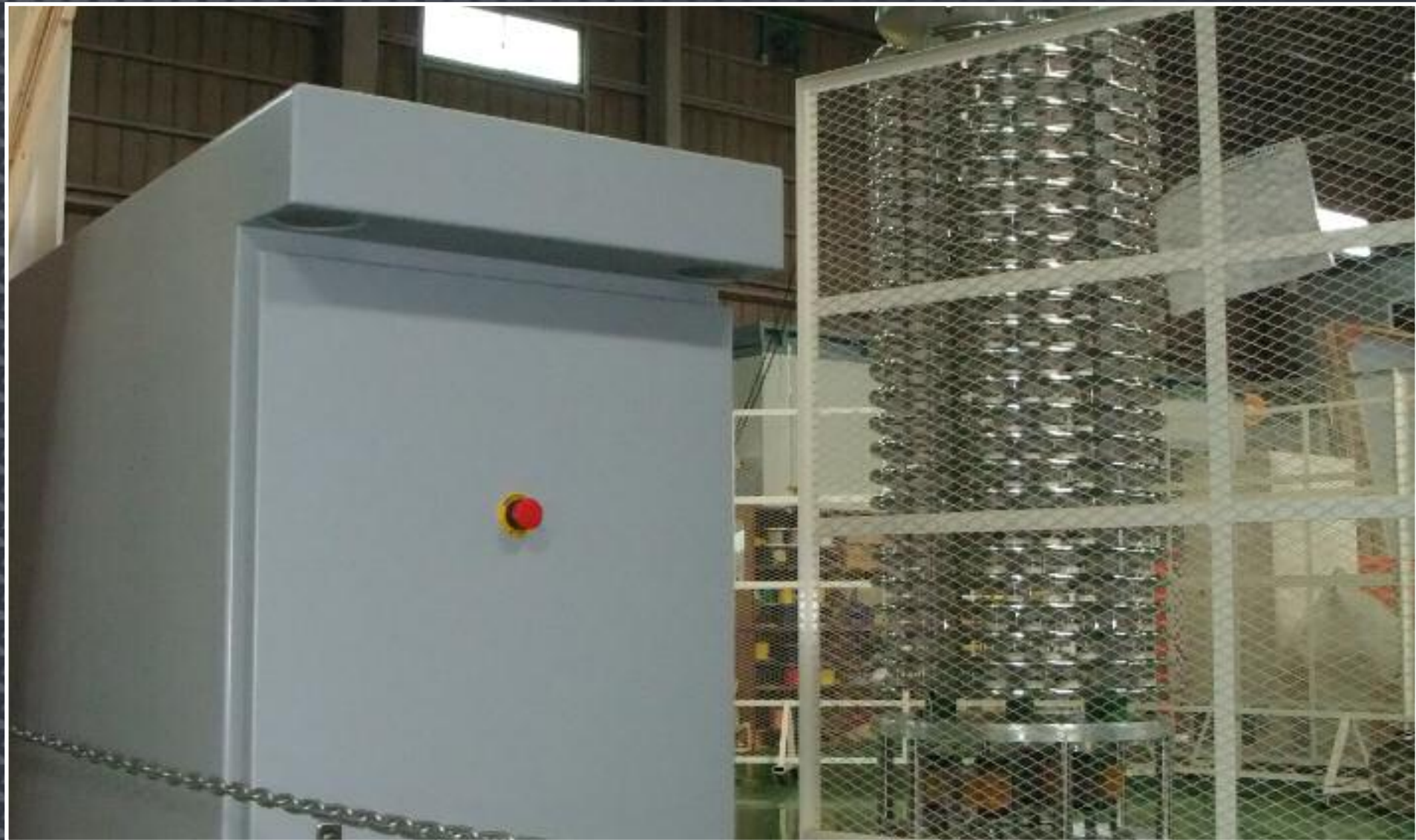
Right-hand side: The cockcroft-Walton electrical circuit to generate 1.3 MV. This is installed in the pressurized tank of the testing power supply. Left-hand side: Invertor to deliver the primary power to the cockcroft-Walton electrical circuit.
