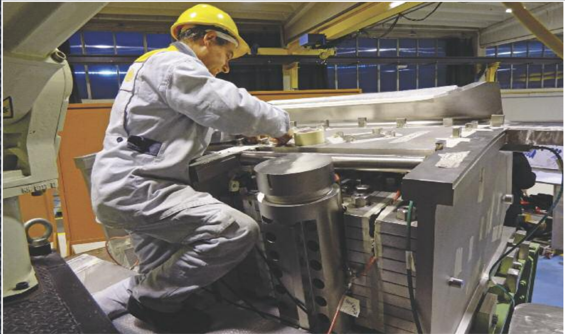
Europe is responsible for seven of the nine sectors that make up the ITER vacuum vessel. A prototype, one-third of the size of the actual component, is currently undergoing bend-testing in Italy. © Walter Tosto
