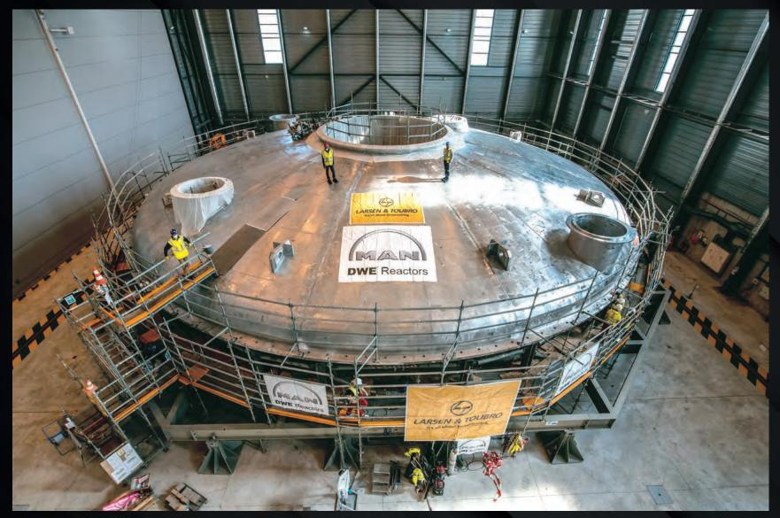
The four sections of the cryostat—base, lower cylinder, upper cylinder and top lid—have been successively assembled and welded in India's Cryostat Workshop. With the top lid finalized (photo), the ITER community can celebrate the completion of a decade-long industrial adventure.
