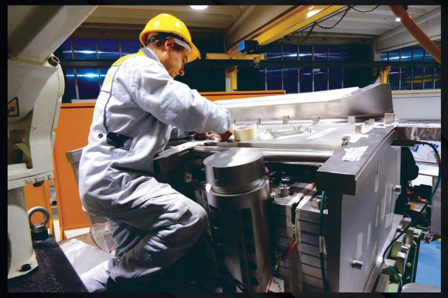
A vacuum vessel prototype, one-third the size of the actual component, undergoes bend testing in Italy. Europe is responsible for five of the nine ITER vacuum vessel sectors.
