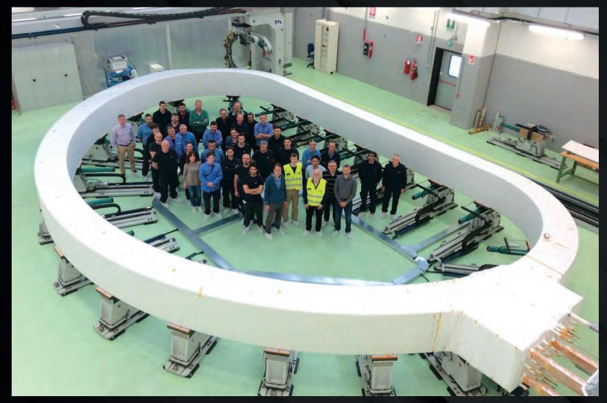
D-shaped toroidal field coils will create the magnetic field that confines the ITER plasma. Europe has successfully completed its first winding pack - the central superconducting core that will be inserted into a structural case.
