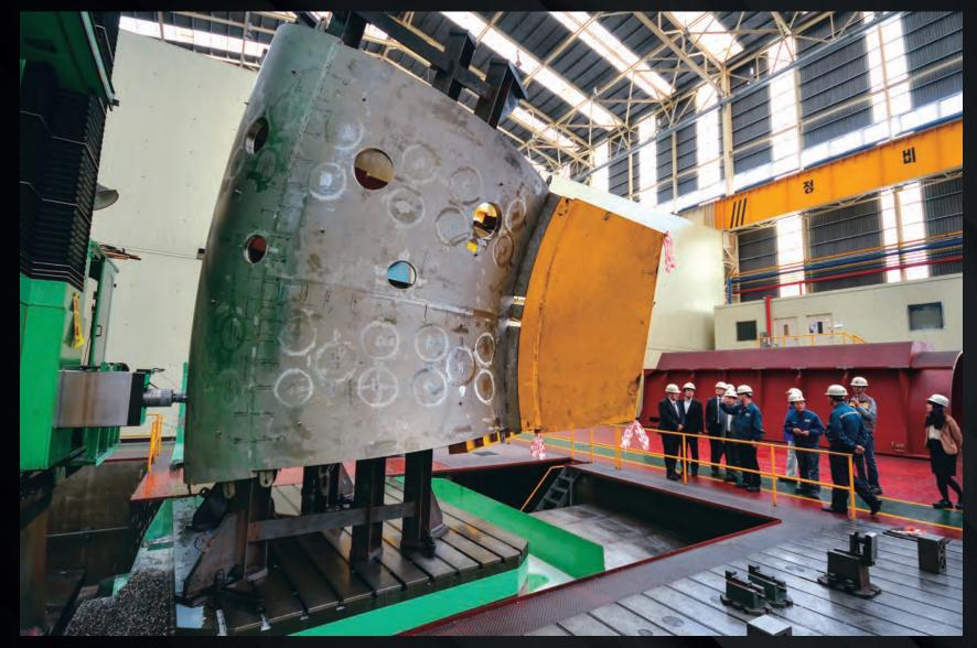
Vacuum vessel fabrication is also underway in Korea, which is responsible for procuring four of the nine sectors. Pictured: welding operations are carried out at Hyundai Heavy Industries in Ulsan on a small part of one sector.
