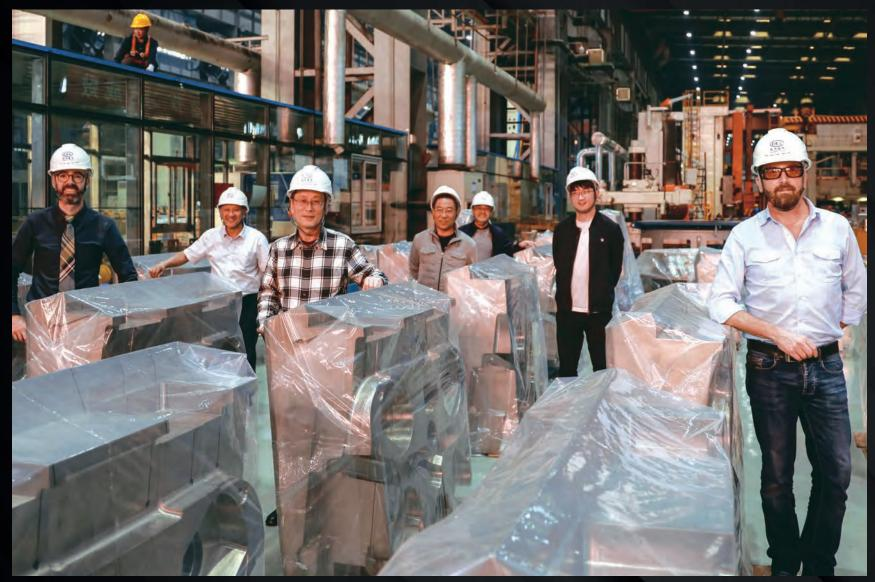
In Korea and in China, where blanket shield block procurement is underway, approximately 55 percent of fabrication is now complete. In this photo, 3-tonne shield blocks are inspected during a progress meeting at Dongfang Heavy Machinery, China.
