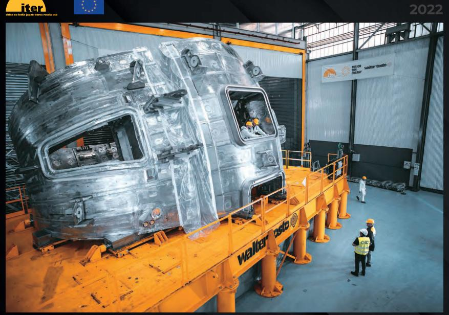
Each vacuum vessel sector is assembled from four smaller segments. In this photo of Europe's sector 4, we can see two segments coming together.
