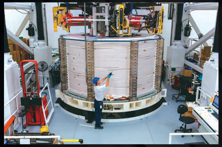
Following heat treatment, the first of six independent magnets for ITER's central solenoid has successfully passed the turn insulation phase at the General Atomics Magnet Technologies Center near San Diego, California. The 1,000-tonne central solenoid, formed from six stacked modules, will "beat" from the very heart of the ITER machine.
