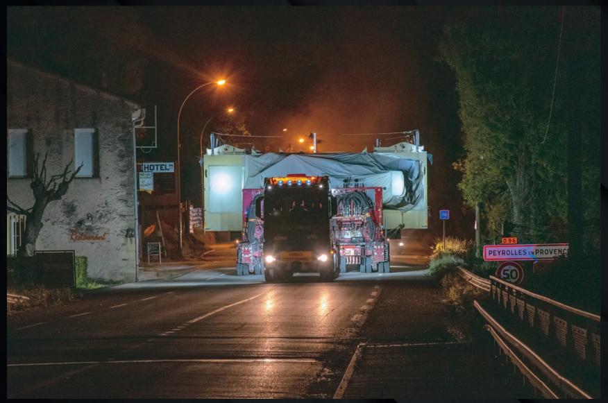
Transport company Mammoet, operating as a contractor to ITER global logistics provider DAHER, has developed a prototype trailer whose twin "power packs" deliver the horsepower equivalent of six conventional truck tractors. It will be used for all of ITER's heaviest loads along the ITER itinerary (pictured, toroidal field coil TF12 from Japan).
