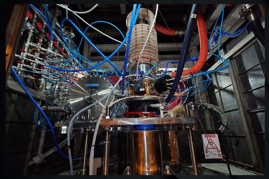
FAT of last gyrotron (one of 8 JADA procured gyrotron) has finished at Naka Institute in QST. Twenty successive shots with 300sec. pulse width / 1MW output power / 50% electrical efficiency is achieved without any failure. It is one of the FAT test items for demonstration of the high reliability.
