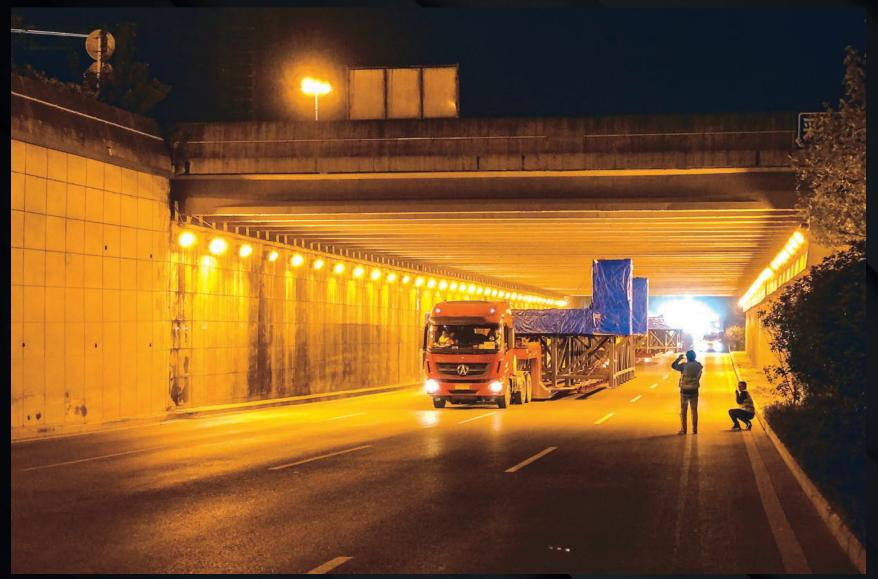
Several large semi-circular components have been delivered for the magnet feeder system that will transport cryogens and electrical power to the bottom correction coil magnets. The feeder sections seen travelling here will be installed inside the cryostat base.
