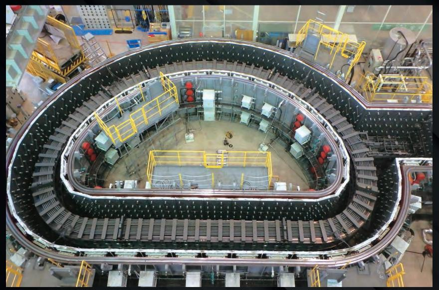
Toroidal field coil windings must be heat treated at 650 °C for 100 hours to react tin and niobium and form the superconducting compound Nb3Sn. In this furnace at Mitsubishi Heavy Industry's Futami factory, seven toroidal coil windings have been successfully heat treated.
