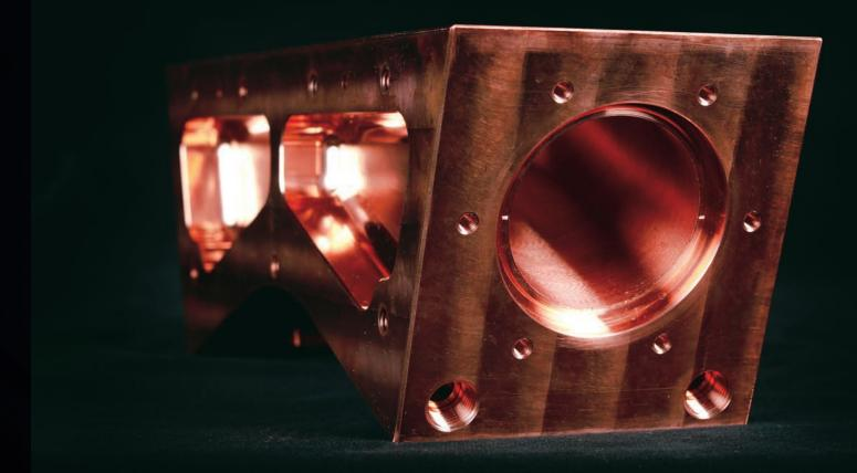
This "mitre bend" waveguide prototype is part of the electron cyclotron transmission lines that will route microwave beams from the Radio Frequency Building to the tokamak, where they will deliver 20 MW of heating power to the ITER plasma. Transmission line R&D, design and fabrication is under the responsibility of the US Domestic Agency.
