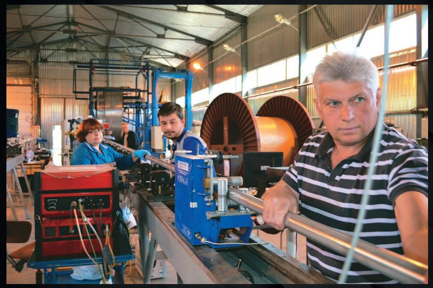
In June, specialists from the Cable Institute (JSC VNIIKP) jacket and compact the last production length of Russian toroidal field conductor at the Institute of High Energy Physics in Protvino, Russia. This milestone marks the end of a five-year campaign to manufacture 28 production lengths, amounting to more than 120 tonnes of material.
