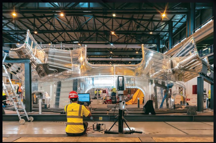
A repair program is underway to replace all thermal shield cooling pipes after analysis showed instances of stress corrosion cracking. Once repaired or re-manufactured, vacuum vessel thermal shield panels like this one will be reassembled with vacuum vessel sectors and toroidal field coils to form the modules that constitute the doughnut-shaped plasma chamber.
