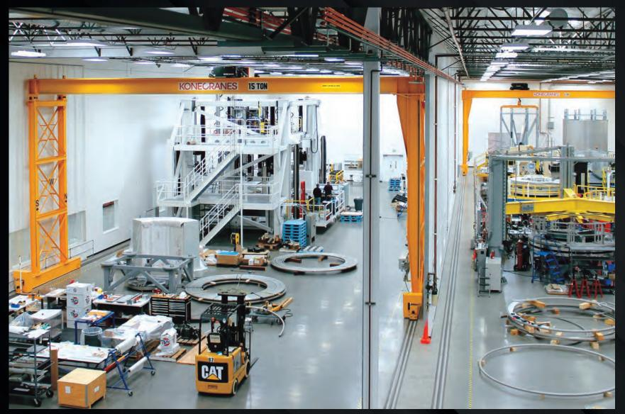
The US central solenoid winding line is inaugurated in April 2015 at the General Atomics Magnet Technologies Center in Poway, California. Winding activities have begun on the magnet packs for the six central solenoid modules plus one spare.
