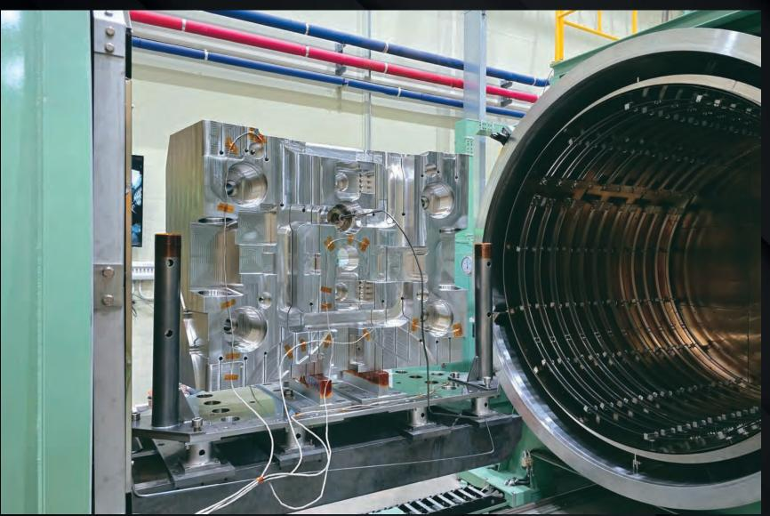
Thick steel blanket shield blocks covering the inner surface of the ITER vacuum vessel will absorb most of the radiative and particle heat fluxes from the hot plasma and stop or slow down the neutrons that result from the fusion reactions. Its complex shape—full of gullies, channels, gaps, and cutouts—has been challenging to manufacture. Here, a shield block is prepared for hot helium leak testing at Vitzrotech, Korea.
