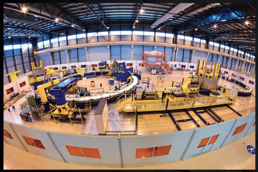
Four of ITER's six ring-shaped poloidal field coils will be manufactured by Europe in this on-site facility, where tooling and process qualification is underway.
