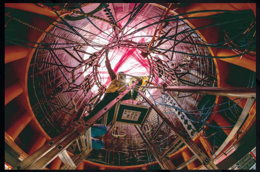
Six independent magnet modules will be stacked to form the central solenoid. The first one, whose helium input pipes and electrical connections are seen here from below, has been positioned on a dedicated assembly platform in the Assembly Hall.
