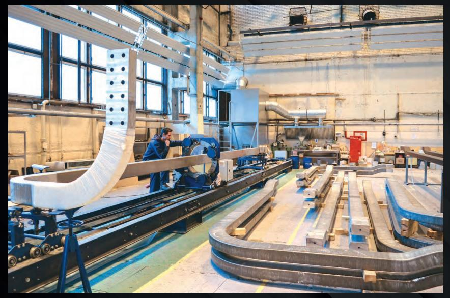
The first batches of these large water-cooled DC busbars, which will feed power to ITER's superconducting magnet coils, have already been received at ITER. Russia's Efremov Institute is manufacturing and shipping 5.4 km of these high-tech components for a total weight exceeding 500 tonnes.
