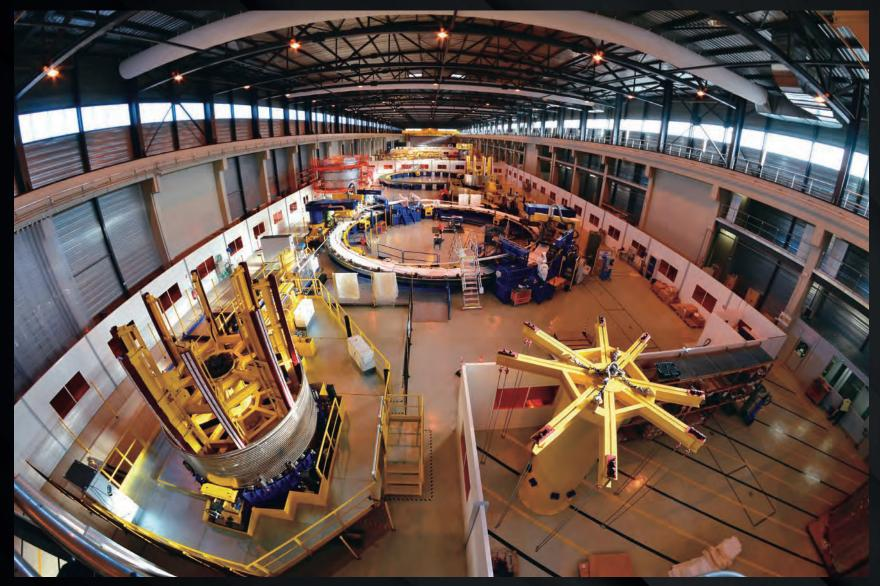
Fabrication has begun on poloidal field coil #5 in Europe's on-site manufacturing facility, after all tooling and process qualification activities were completed. PF5 measures 17 metres in diameter.
