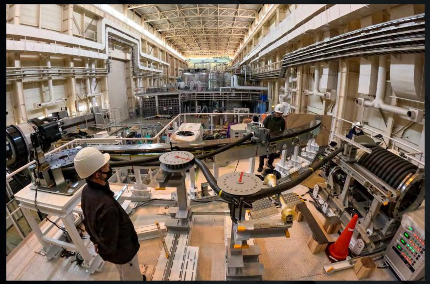
Captions ITo develop composite cable feeding control technology and cable guide mechanism for cable handling equipment, a mock-up test rig was fabricated and completed on March 31, 2023. Test is currently ongoing to reflect the results to the design.
