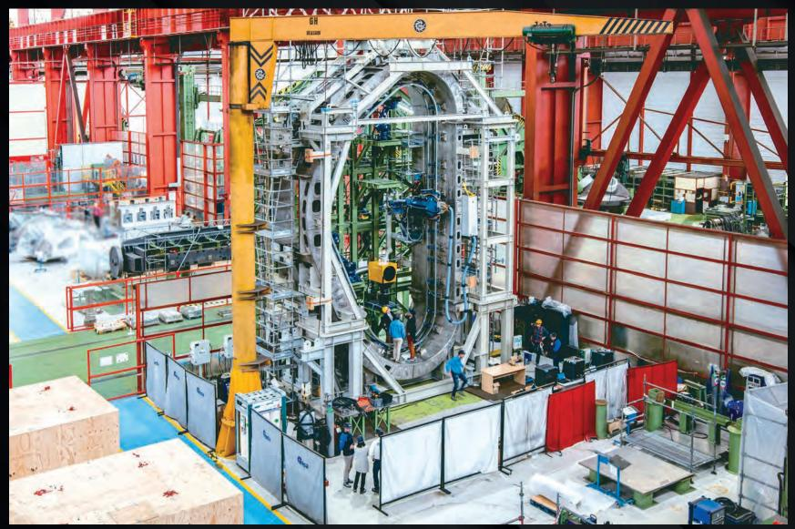
This mock-up of an ITER vacuum vessel sector stands as high as a five-storey building in ENSA's special projects workshop in the outskirts of Santander, Spain. With the exception of sector width (10 degrees versus 40 degrees) it mirrors the future reality of ITER down to the smallest detail. It will be used to develop and test welding tools.
