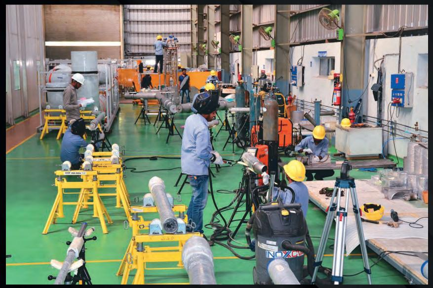
Procurement for the ITER cryolines—the highly sophisticated multi-process pipes that transport cooling fluids—is shared by France's Air Liquide and India's INOXCVA (pictured here). ITER will have approximately 5 kilometres of cryolines ranging from 25 to 1000 millimetres in diameter.
