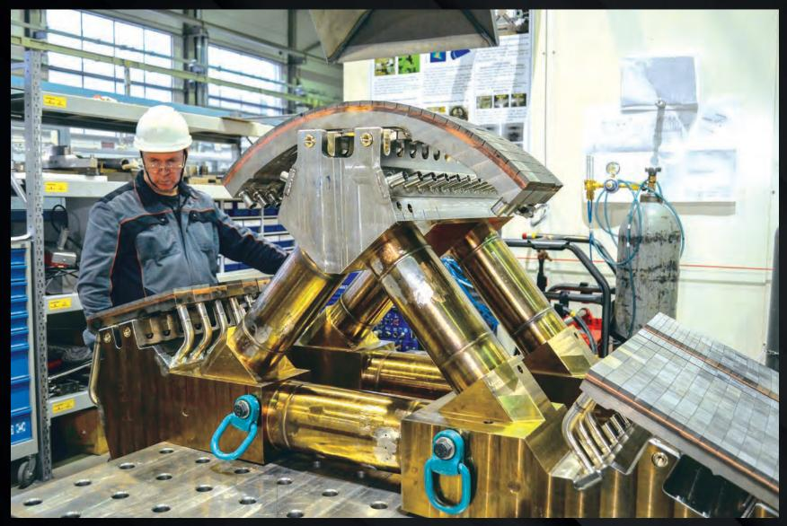
The Russian Federation has completed the first full-scale prototype of the divertor dome. One of three divertor targets designed to sustain the top heat flux of the ITER machine (10 to 20 MW/m²), a dome component will be mounted on each of the 54 divertor cassettes.
