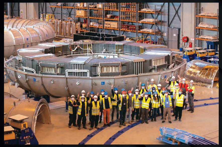
The first poloidal field coil completes all testing in December. Representatives of the European Domestic Agency Fusion for Energy, manufacturer ASIPP from China, and ASG Superconductors celebrate in front of the vacuum chamber where poloidal field coil #6 spent three months in thermal testing.
