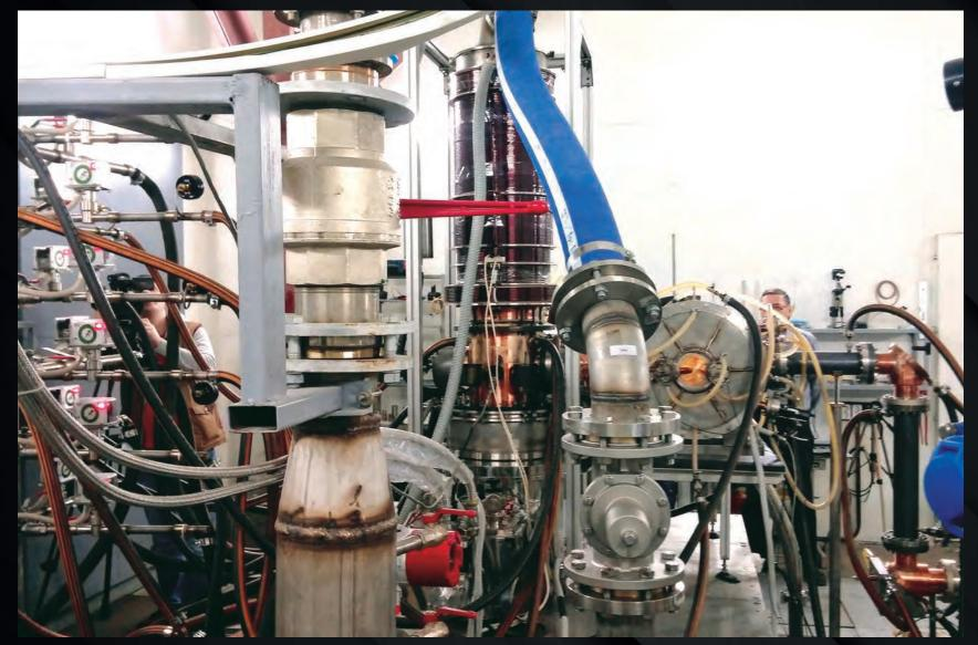
A gyrotron prototype successfully passes factory acceptance tests at Gycom Ltd in Nizhny Novgorod, Russia. These energy-generating devices will inject powerful microwave beams into the ITER vacuum vessel to heat the plasma and drive plasma current.
