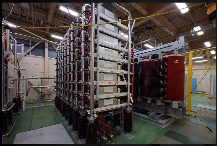
Modern PSM high power supply for gyrotron operation was introduced in QST for imitate the ITER gyrotron power supply. The stable beam current operation was confirmed with JADA gyrotron. The operation parameter by using PSM power supply is learned for ITER Sight Acceptance Test (SAT).
