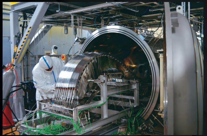
This divertor outer vertical target prototype manufactured by Mitsubishi Heavy Industries in Japan prepares to enter hot helium leak testing. The validation phase of this critical plasma-facing component has almost concluded; series manufacturing comes next.
