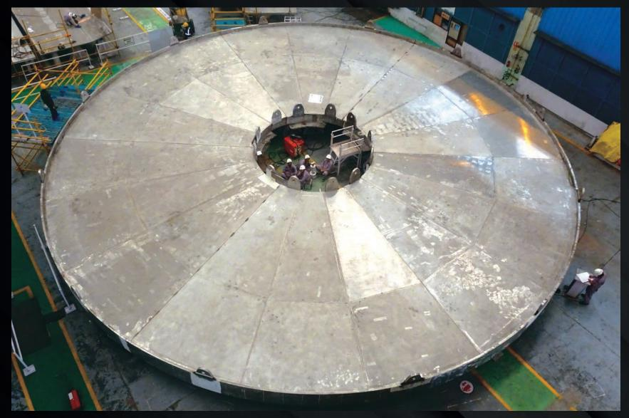
At the Larsen & Toubro Ltd factory in Hazira, India, Tier 1 of the cryostat base is assembled on the shop floor to verify tolerances before being shipped in six 60° segments to the ITER site. The cryostat base is the heaviest single component of ITER assembly (1,250 tonnes).
