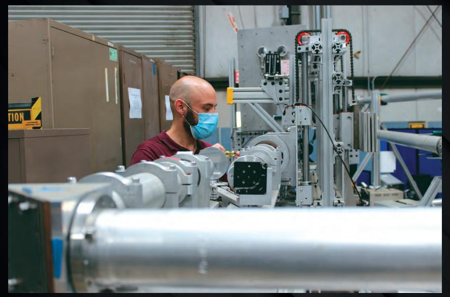
Prototypes for the low field side reflectometer diagnostic are in development at General Atomics. This diagnostic system will monitor electron density and aid in the assessment of fusion performance.
