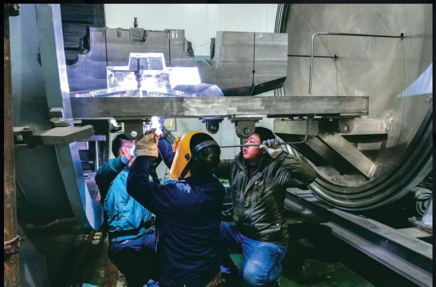
Hot helium leak tests on this 2.8-tonne blanket shield block prototype have successfully confirmed its suitability for ITER's ultra-high vacuum environment.
