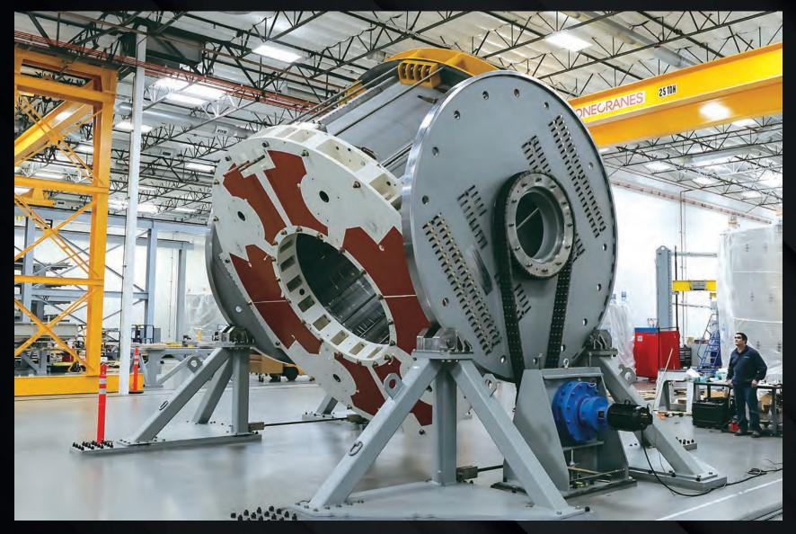
At different stages of fabrication, the top or bottom of a central solenoid module must be accessible. This turnover tool at General Atomics (California) makes easy work of flipping the 110-tonne components.
