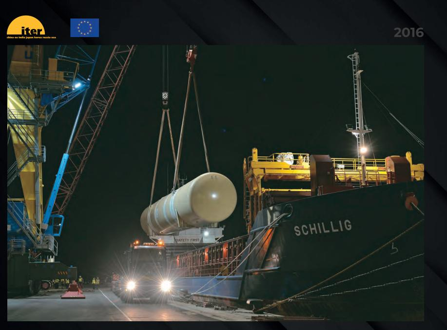
Large components like this cryoplant tank procured by Europe are shipped by sea to the Mediterranean port of Fos-sur-Mer before continuing along a specially adapted road itinerary to the ITER site.
