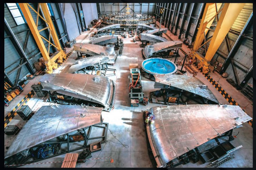
The segments of the cryostat lid arrive early in the year from India. They will be assembled and welded on the platform at the far end of the Cryostat Workshop.
