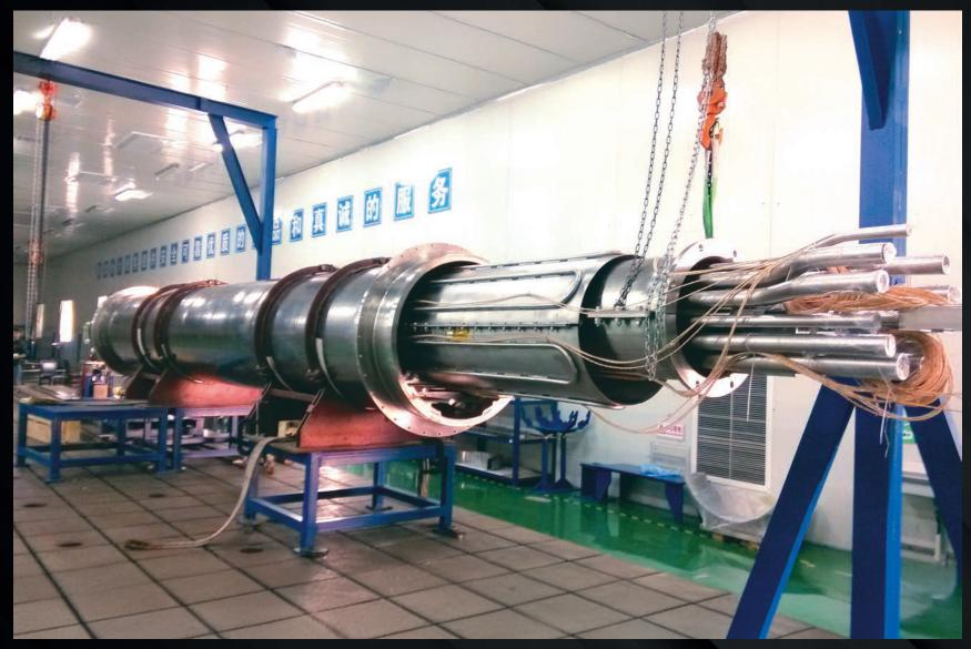
Cryostat feedthroughs cross through the cryostat and bioshield to provide a passageway to the ITER magnets for cooling pipes, power and instrumentation cables. This 10-metre prototype was manufactured at the Institute of Plasma Physics, Chinese Academy of Sciences (ASIPP).
