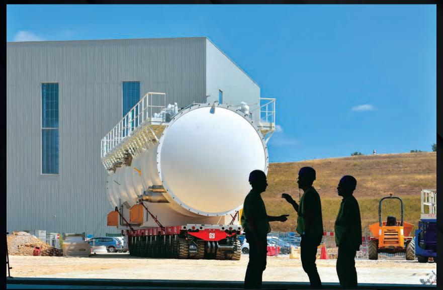
Manufactured in France by Air Liquide, this helium "cold box" – installed with two others in the cryoplant during the year – will provide insulation for the key components of the liquid helium plants.
