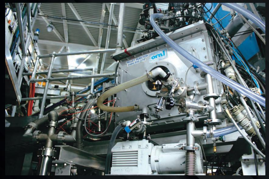
The plasma will be fed frozen pellets of fuel, fired into the vacuum vessel by pellet injectors. Here, a pellet injector developed by Oak Ridge National Laboratory is installed on the DIII-D tokamak (San Diego, California) for testing.
